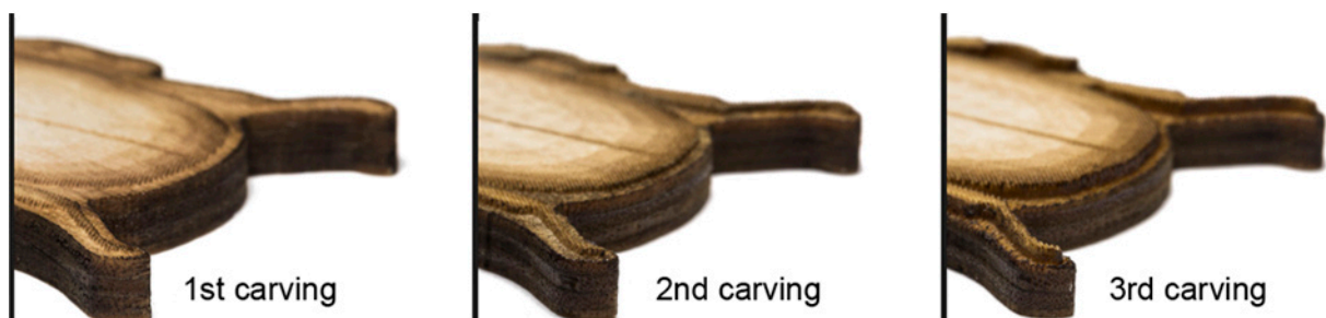
Figure 5. Example of carving three times with the same power on the same area.
