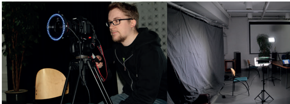
Figure 3. Chromatte LED ringlight in camera and chromatte screen (Photos: Mikko Shemeikka)
