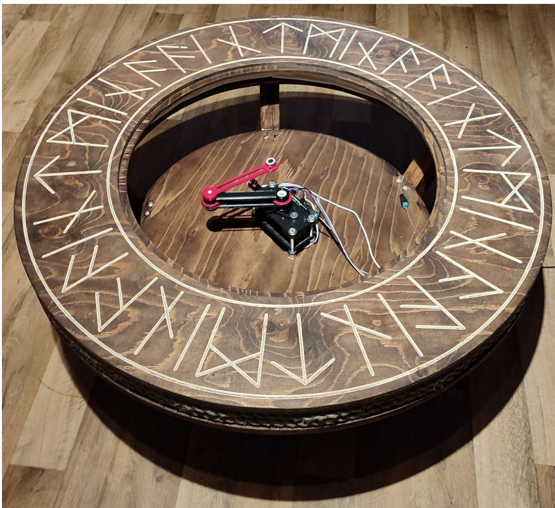
Illustration 7: Robotic arm inside the table
