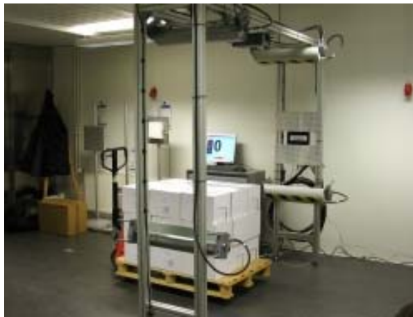
Picture 1. An RFID reader is able to read/write data from/on an RFID tag by using radio signals. (Vilant Systems Oy:272)
