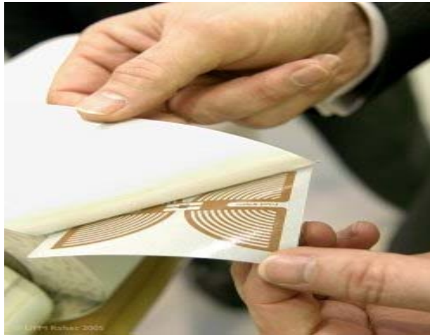
Picture 3. Passive RFID tags contain no battery, and are often in the form of a shipping label. The read distance of passive tags is less than 10 meters. (Vilant Systems Oy:272)
