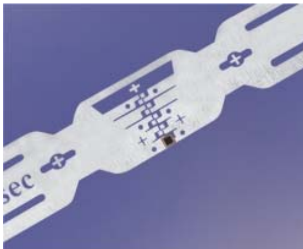
Picture 2. The information is stored on the RFID chip of the RFID tag. (Vilant Systems Oy:272)
