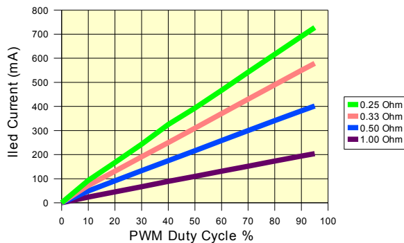
Mean LED current vs. PWM duty cycle at a PWM frequency of 500 Hz at different values of Rsense.
