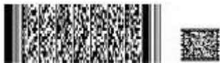
FIGURE 2. Space requirements for the PDF417 (left) and CM (right) when saving 200 numbers
