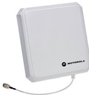
Kuvio 6. RFID- antenni (Strategic Systems & Technology Corporation 2015)
