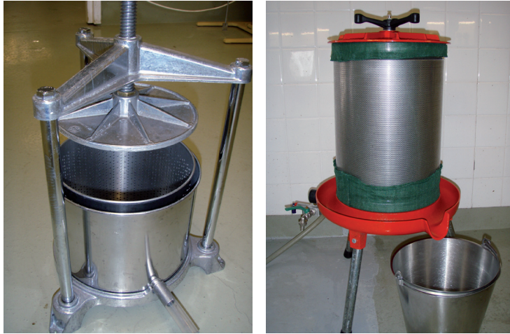
Figure 6. 4.5 l juice press (Palumbo) used for pressing currants (left) and 40 l hydraulic pressure juicer (EPL 740) used for apples.
