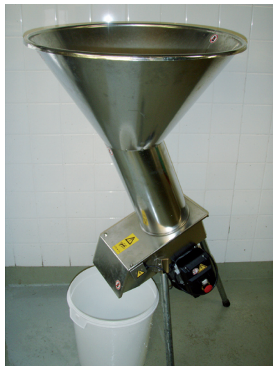
Figure 5. Apple crusher (EPL 23 Mixer, Enotecnica Pillan).
