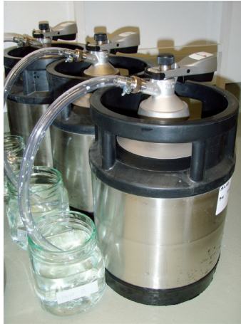
Figure 7. Ten-litre steel vessels (Das Finn-Keg) used for the fermentation and aging of apple and currant wines.
