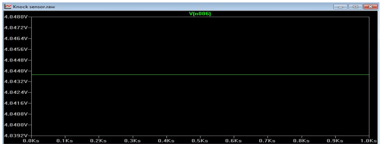
Figure 26 - Diagnostic voltage when a "bad" sensor is simulated
