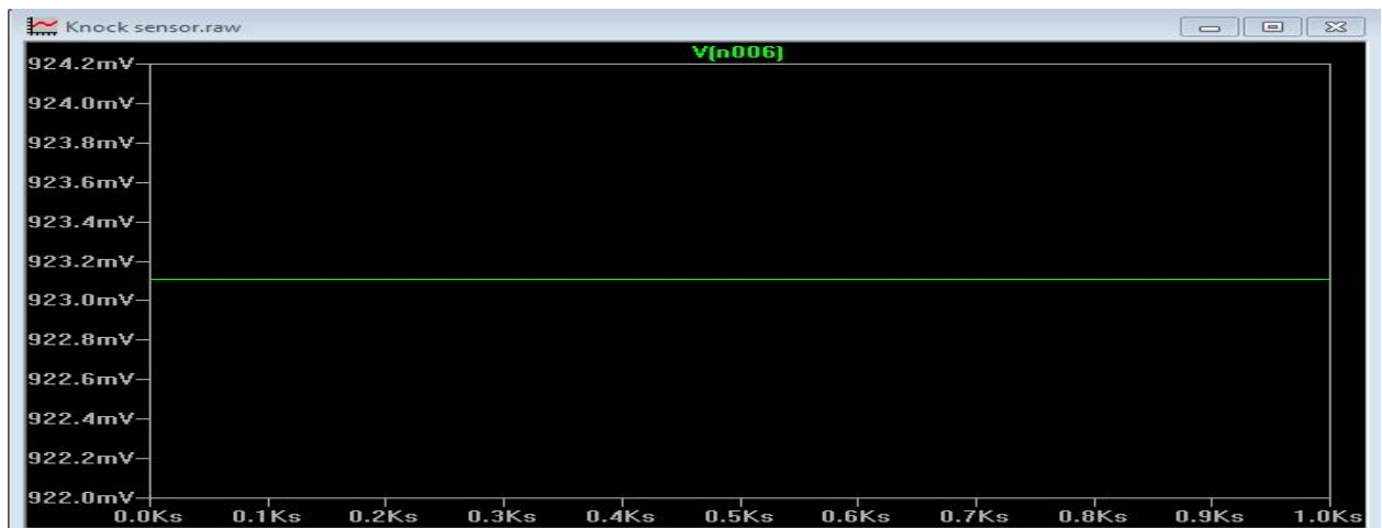
Figure 24 - Diagnostic voltage when a “good” sensor is simulated
