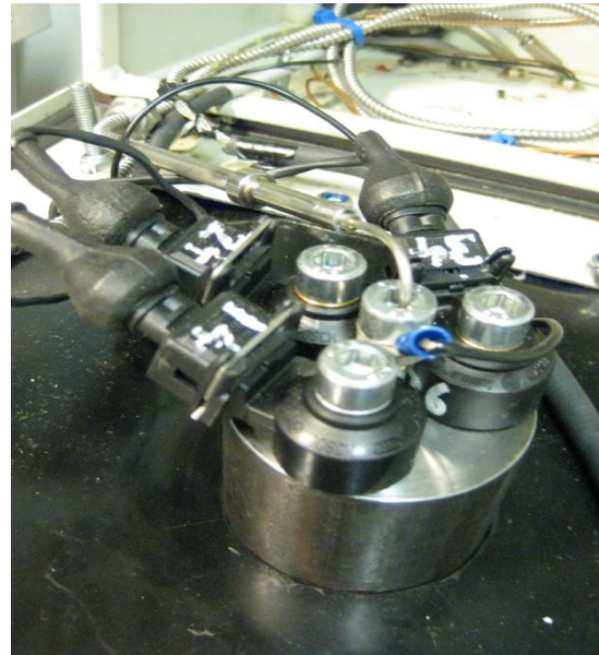
Figure 21- Knock sensors mounted in the heat /vibration cabinet
