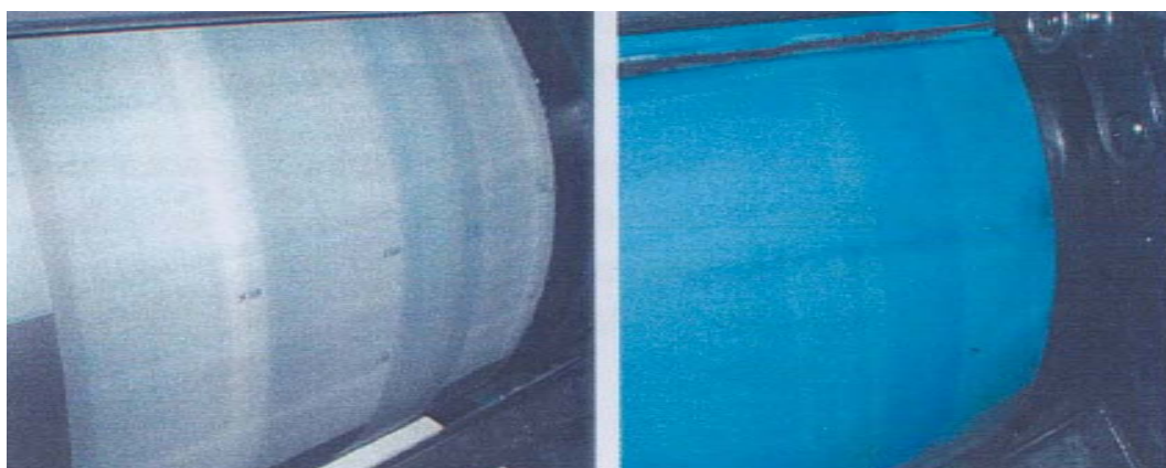
Figure 3 On the left a blanket after 30,000 copies and on the right the same blanket after washing /11/
