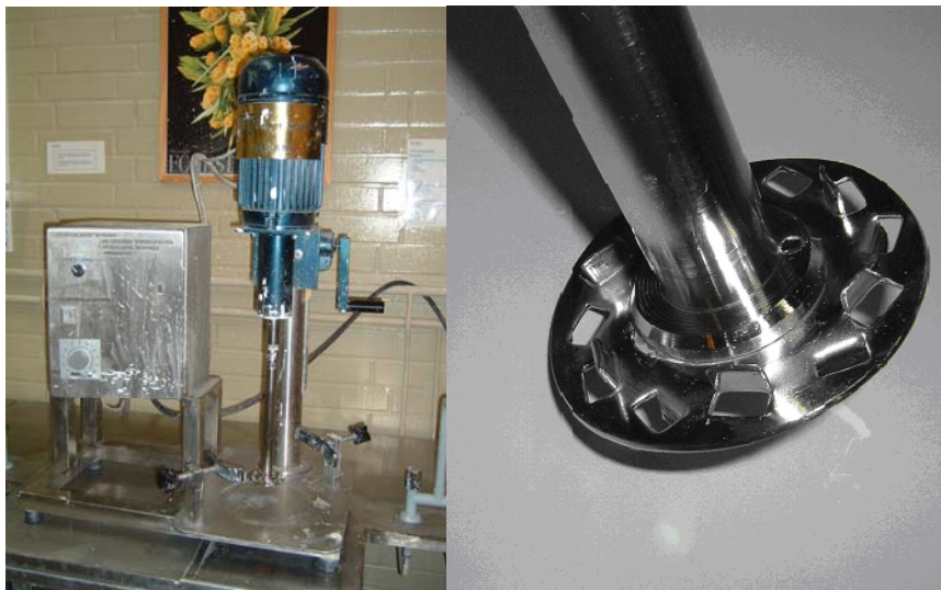
Figure 3 Mixer and impeller details
