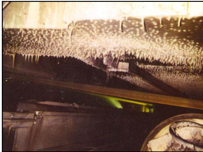
Picture 1 Growth of slime in paper machine /9/
