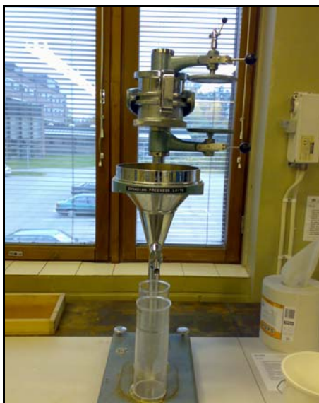
Picture 15 Canadian Standard Freeness measuring equipment
