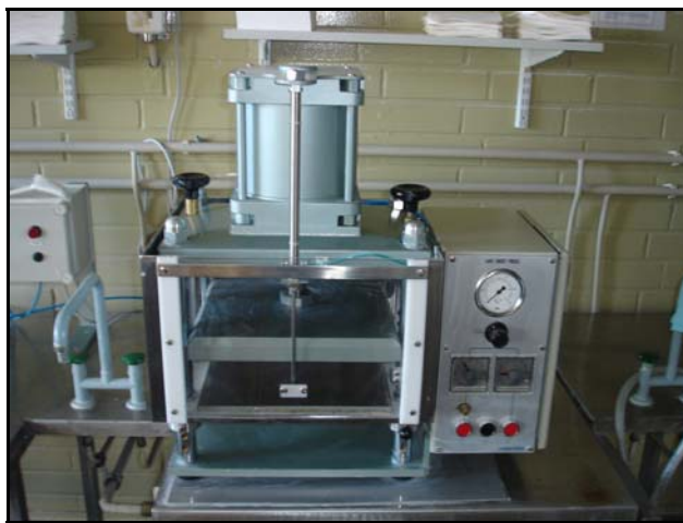
Picture 13 L&W Sheet Press machine
