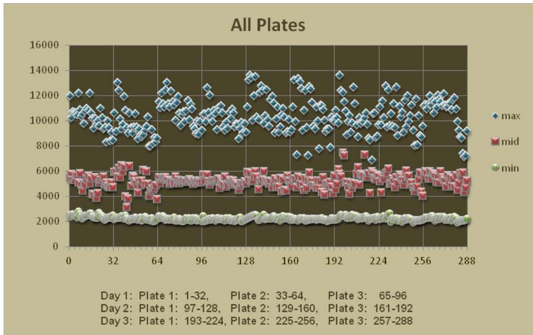
Figure 32. Signal Variability, All Signal Levels. Each plate is plotted against fluorescence intensity [FI].
