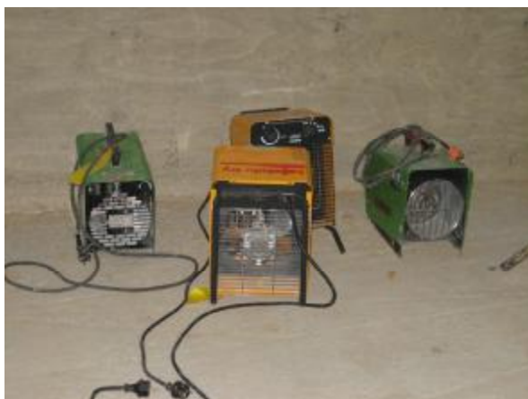
Img. 522. Gas burning heater fans
