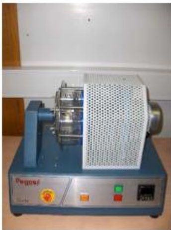
Figure 36 : Water vapour permeability tester machine
