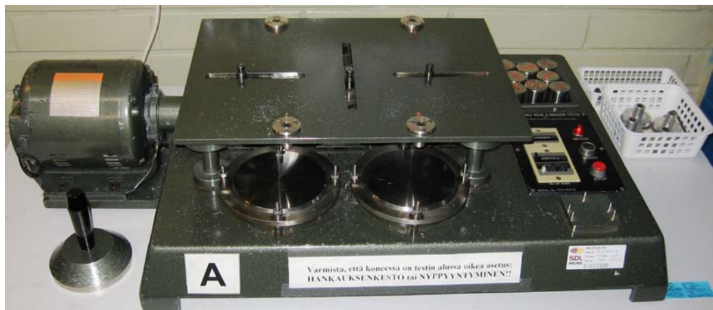
Kuva 2 James H. Heal & Co. (Martindale wear and abrasion tester)
