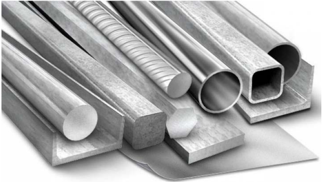
Figure 2.5. Different types of the rolled sections
