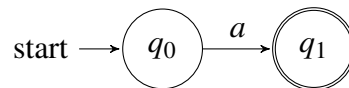
FIGURE 17. An automaton resulting from conversion of a using the Thompson's construction algorithm
