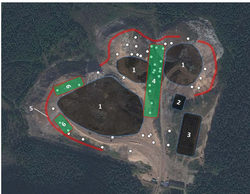
Figure 2. The site plan of the municipal solid waste landfill No. 1 with an indication of sample collection points: 1 – the operated areas, 2 – the repository of hazardous waste, 3 – the building area, 4 – the preferable area with high methane concentration for biogas potential usage, 5 – the areas of wastes combustion, 6 – the areas with high methane concentration
