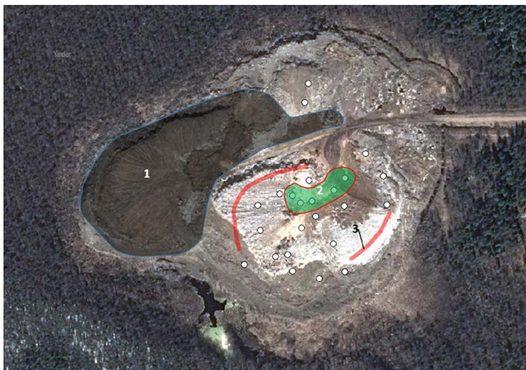
Figure 3. The site plan of the municipal solid waste landfill No. 2 with an indication of sample collection points: 1 – the operated area, 2 – the preferable area with high methane concentration for biogas potential usage. 3 – the areas of wastes combustion
