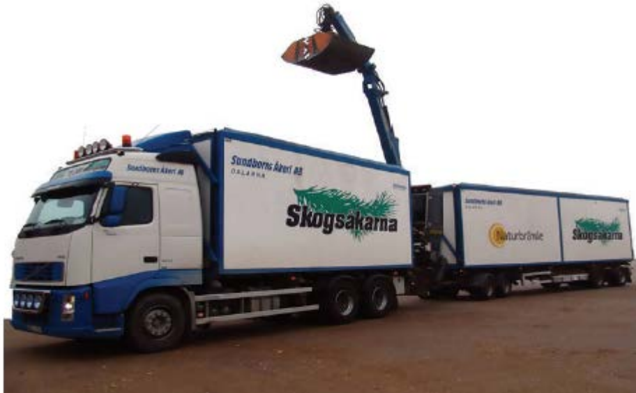
Figure 18. Self-loading chip truck in Sweden equipped with a bucket for loading of wood chips. (Source: Mortazavi & Johansson 2013).
