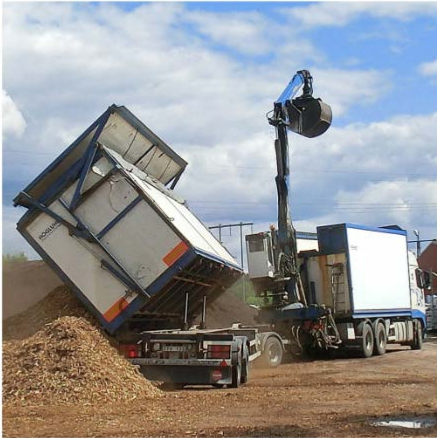
Figure 17. A chip truck that uses side tipping system for fuel delivery. (Source: Eriksson, 2014).
