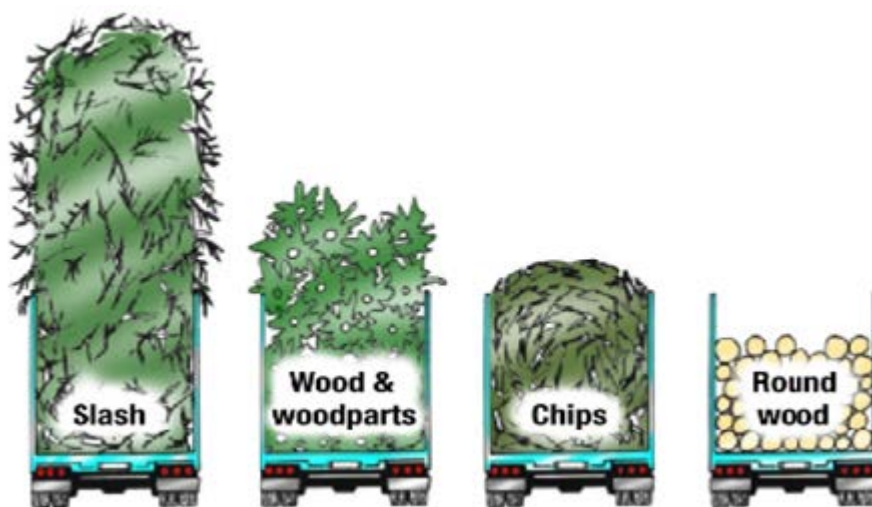
Figure 14. Shows the importance of transportation by representing volume differences of the same weight material by different product types. (Source: Sustainable Forestry for Bioenergy and Bio-based Products).
