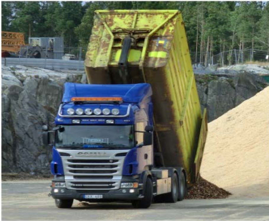
Figure 15. A hook-lift truck emptying a bin. (Source: Eriksson, 2014).
