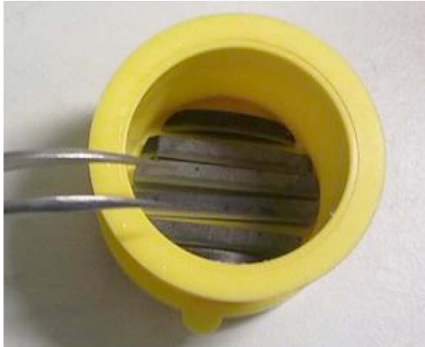
Picture 3. Positioning of sample slices for re-casting.
