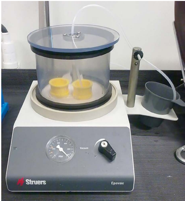
Picture 1. Epovac – Epoxy casting of a sample in vacuum.
