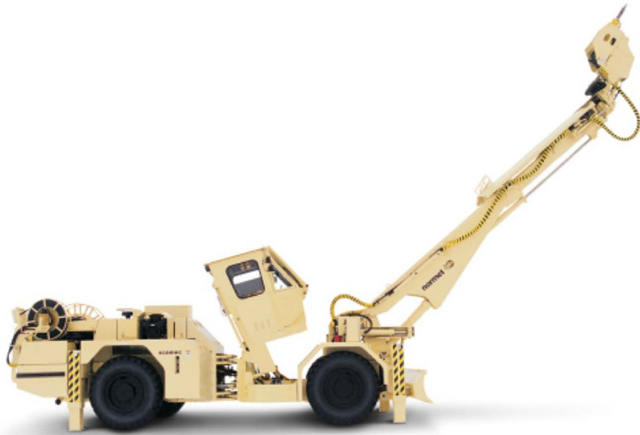
Picture 5. Scaling rig (Normet 2015).
