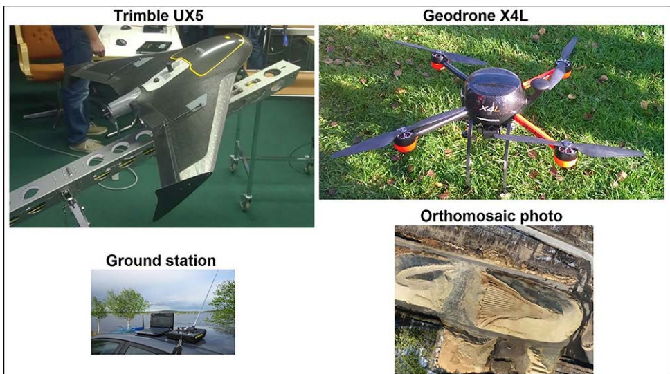
Figure 7. An unmanned aerial system (UAS) is a combination of hardware and software that produces 2D and 3D data and image products, such as digital terrain models and orthomosaic photos.
