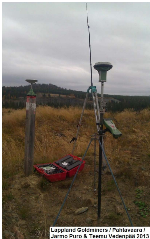
Picture 1. Base and remote receivers for real time kinematic (RTK) survey. The base receiver is at a control point. In the middle can be seen the antenna of the radio modem. From Lapland Goldminers' Pahtavaara Mine. (Puro & Vedenpää 2013.)
