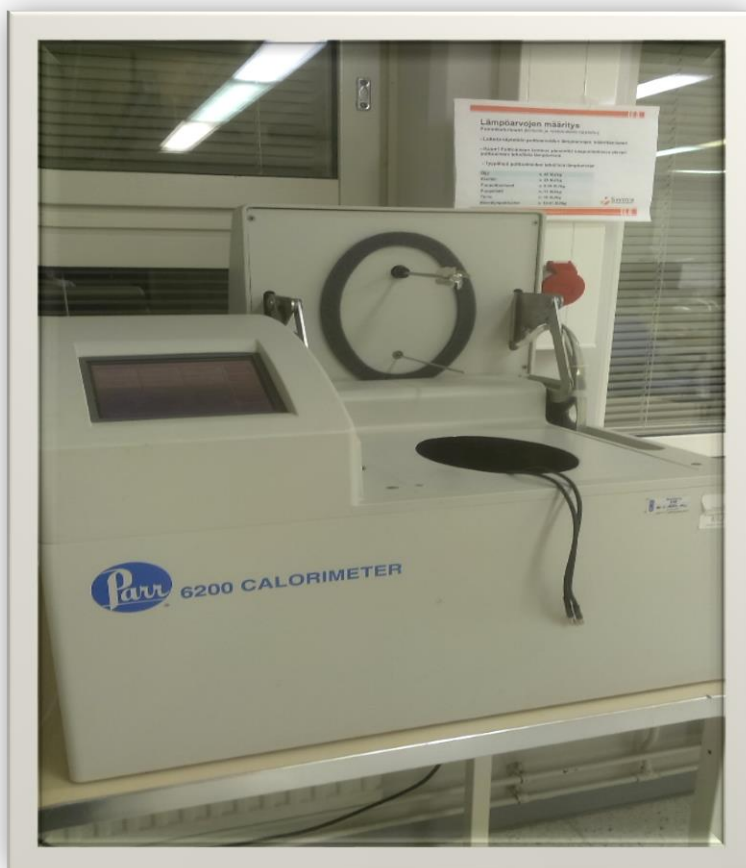
Figure 12. The bomb calorimeter
