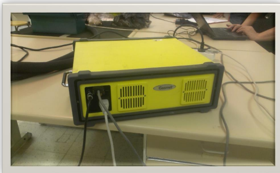
Figure 14. Flue gas content analyzer
