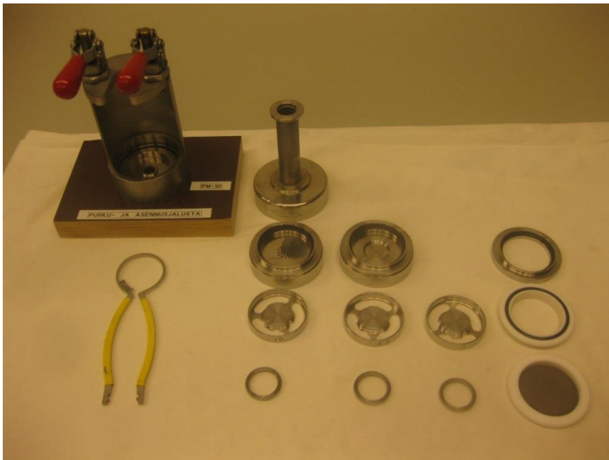
PICTURE 4. The disassembled stages in lines from PM10 stage parts on the left to the filter stage on the right
