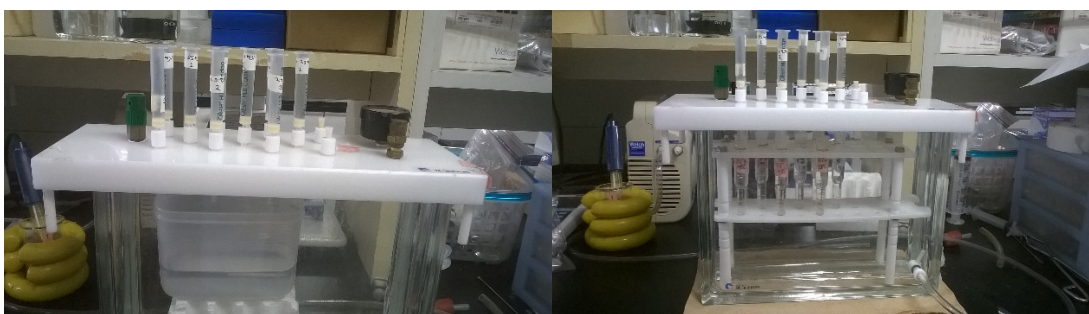
Figure 12. Shows SPE-sample washing and SPE- extraction
