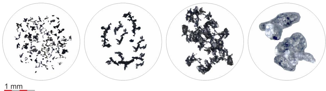
FIGURE 8. VTT's sintering classification from left to right O, *, **, *** (mod. from Moilanen 2006)
