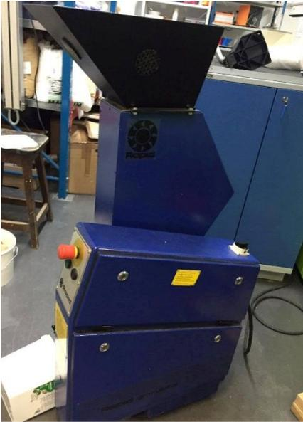
*Figure 10. Rapid shredder*
