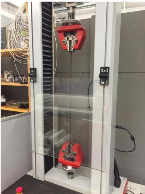
Figure 17. Tensile testing of rHDPE panel
