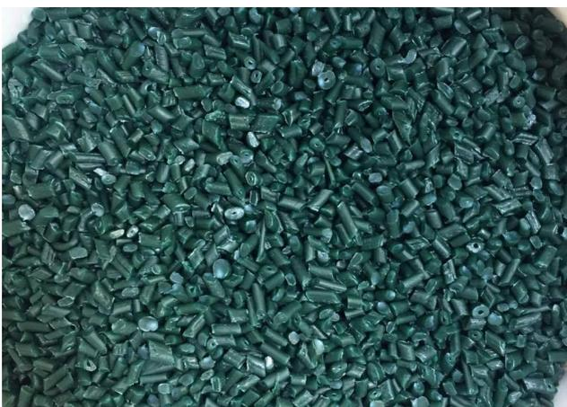
*Figure 13. Pellets of recycled watering pots*
