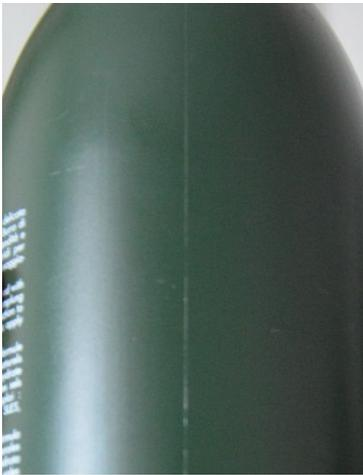
*Figure 7. Thin rim left by the split mold*
