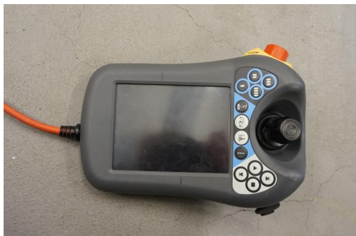
Figure 1-1: The panel board for the ABB IR2600 welding robot
