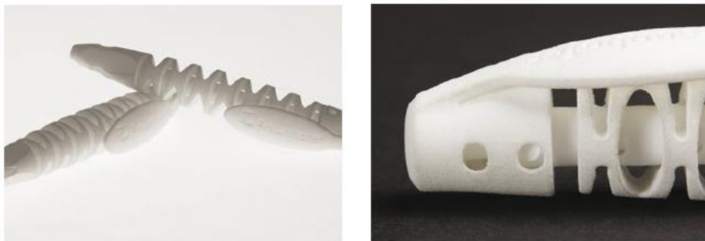
Figure 3-2: A pen produced with additive manufacturing. On the right side the opening for the powder removal is visible (Breuninger et al. 2013, 122)
