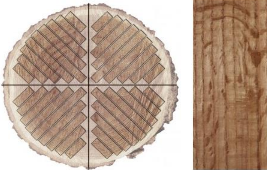
Figure 12. A quarter method of sawing (Sawing Options , n.d.)
