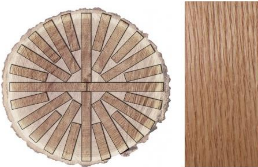
Figure 10. Cut pattern for rift sawn lumber (Sawing Options , n.d.)
