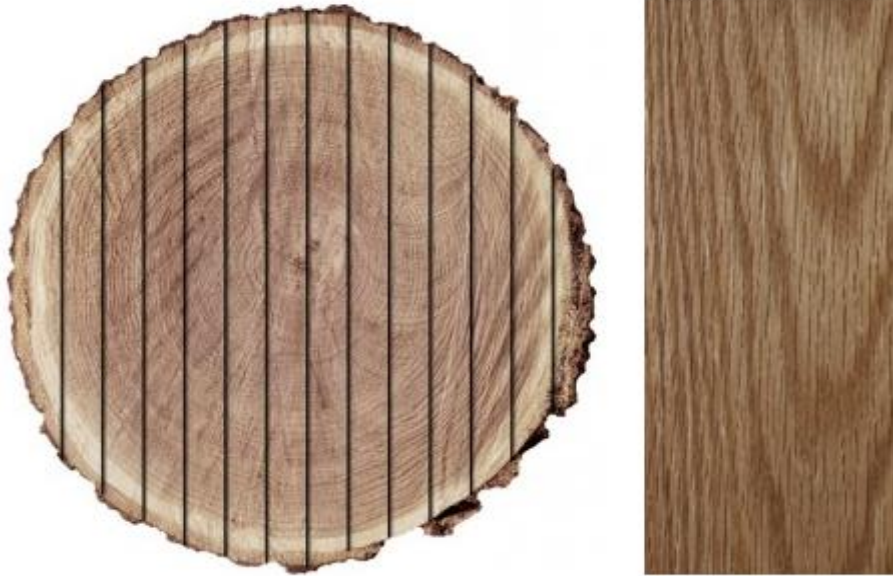
Figure 11. Plain method of sawing (Sawing Options , n.d.)
