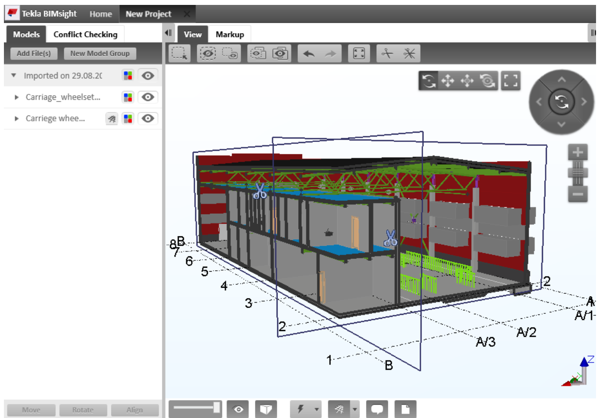
Figure 11. Tekla BIMsight. Checking models' arrangement.
