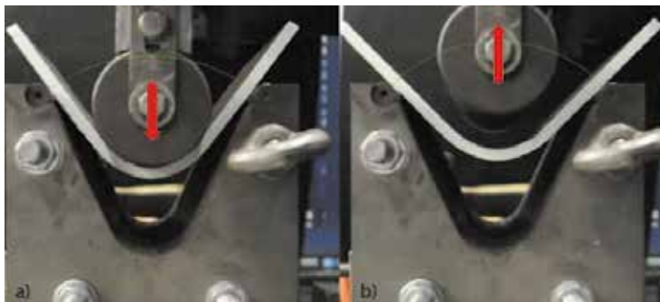
Figure 4. Bending of a steel plate in a V-die: a) punch in lower position; b) punch released
