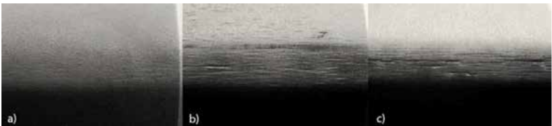
Figure 5. a) No failures; b) and c) failures appeared in the steel as a result of too small a bending radius
