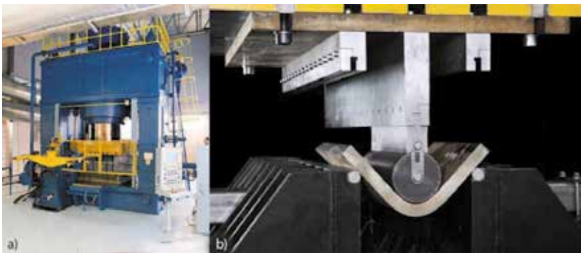
Figure 8. a) Hydroforming machine and b) bending tools built in the machine
