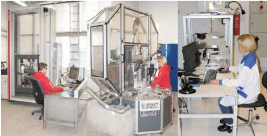
Figure 9. Tensile test, impact test, and hardness test
