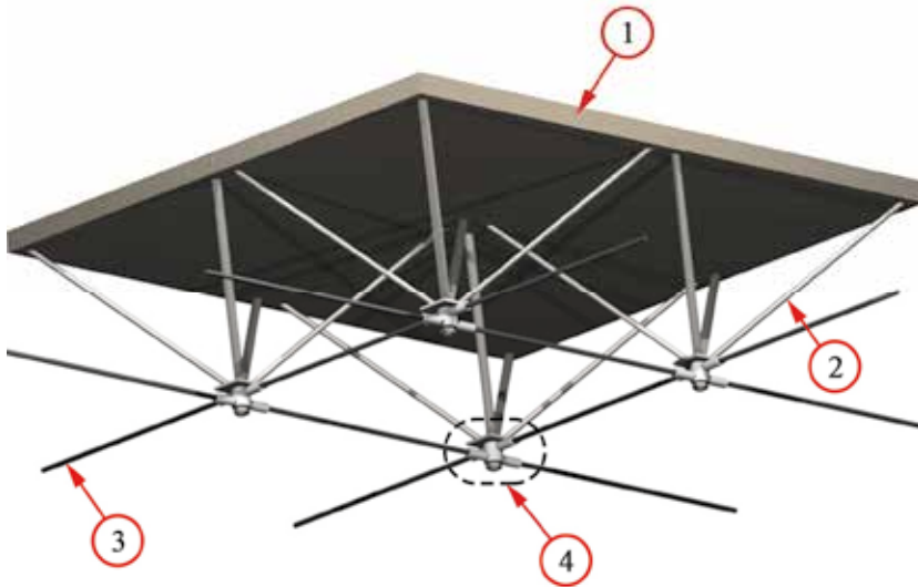
Figure 1. Segment of The flat double-layer grid-cable steel-concrete composite structure: 1 – a top chord; 2 – a diagonal; 3 – a bottom chord; 4 – a nodal bolted connections
