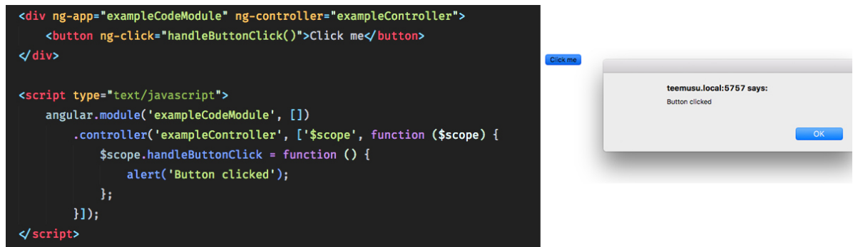
Figure 5. Scope functions can be executed when a user clicks a button in the view. $scope is passed to the controller via dependency injection – a method of providing dependencies to components as requested. A click is registered with a built in ng-click directive.
