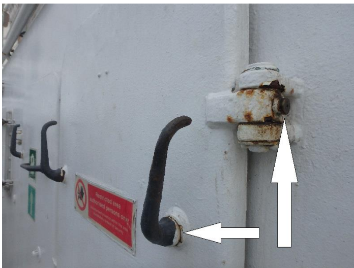
Cargo hold fan crank, stb and bb side
