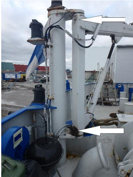
Liferaft light stb and bb side, greasing the rod mounting
