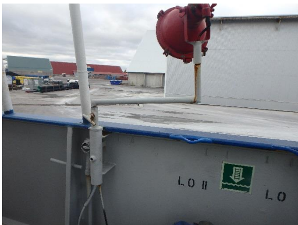
Liferaft light stb and bb side, greasing the rod mounting
