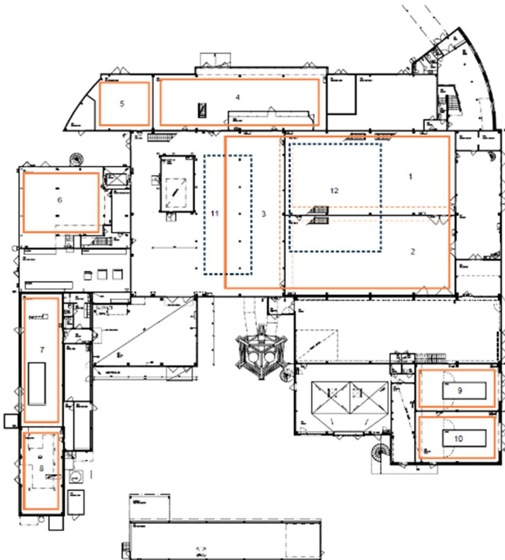
Figure 2. Existing emergency stop areas in the building. Orange lines shows the 1<sup>st</sup>. floor emergency stop areas and blue dotted line the 2<sup>nd</sup>. floor emergency stop areas.
