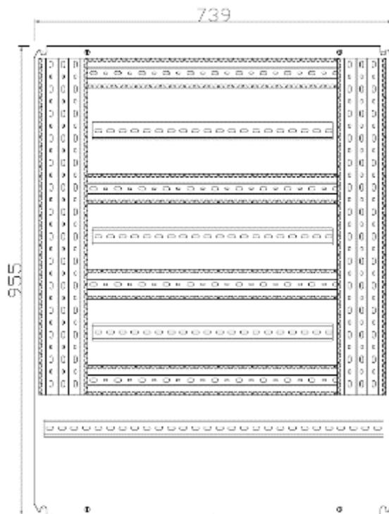
Figure 20. Layout of the DIN-rails and cable ducts on Rittal AE 1180.500 cabin mounting plate.
