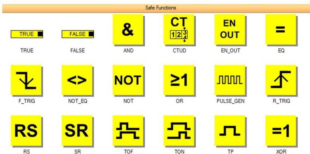
Figure 24. Safety functions available for FBD programming of safety PLC.
