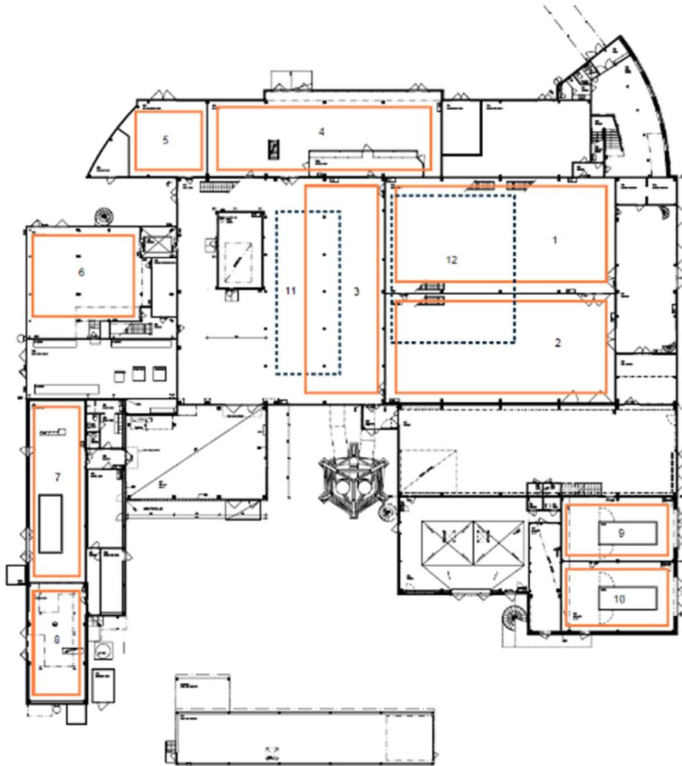
Figure 3. Planned building emergency stop areas. Orange lines shows the 1<sup>st</sup>. floor emergency stop areas and blue dotted line the 2<sup>nd</sup>. floor emergency stop areas. Building consist 12 areas and 12 emergency stop areas.
