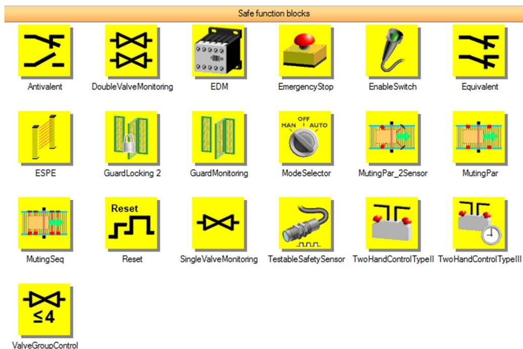
Figure 25. Available safety function blocks for programming.
