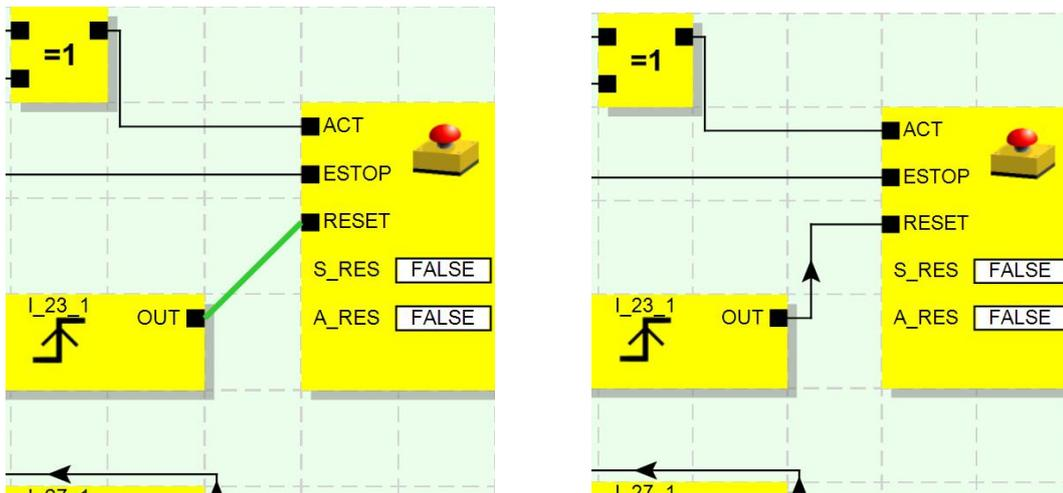
Figure 26 (left). If connection is allowed the straight line appears in green colour. If connection is not allowed line is red and connection is not made. Figure 27 (right). Successful connection.
