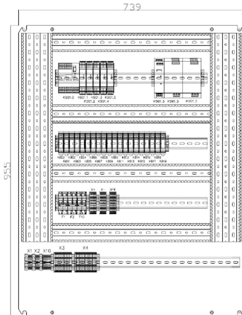
Figure 22. CJU541 layout, slightly different compared to CJU901.
