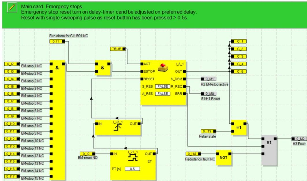
Figure 31. CJU541 area main network. Similarities between common panel and test rig area emergency stop is notable.
