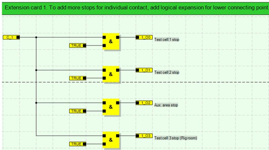
Figure 30. Common panel CJU901 extension card program, each extension card program has its own program network.
