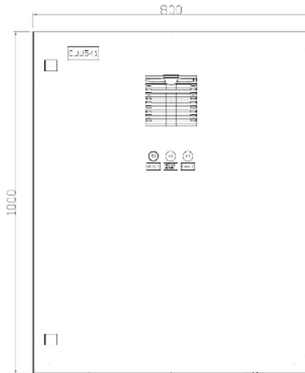
Figure 19. Face layout for emergency stop cabin CJU541. The electrical cabin doors of the emergency stop system are mostly identical.
