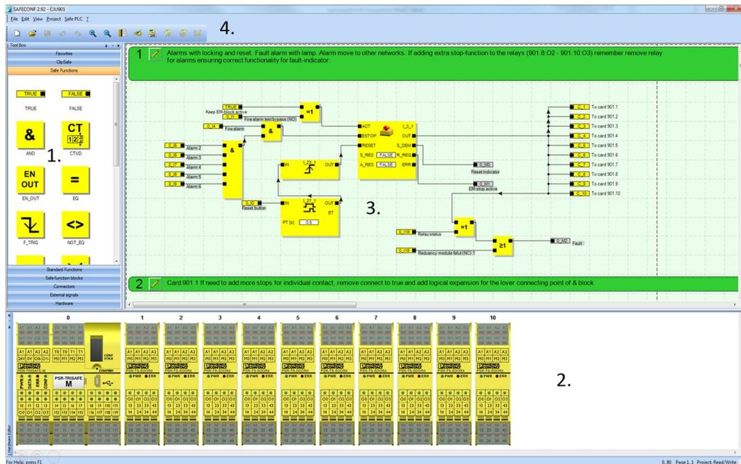
Figure 23. The SAFECONF – main window. 1. Tool Box, drag & drop logical functions for toolbox. 2. Hardware Editor, modify hardware suitable on project and program. Add hardware for toolbox menu with drag & drop. 3. Program Network, add and connect logical functions, inputs and outputs for program network. 4. Menu for properties and tools.
