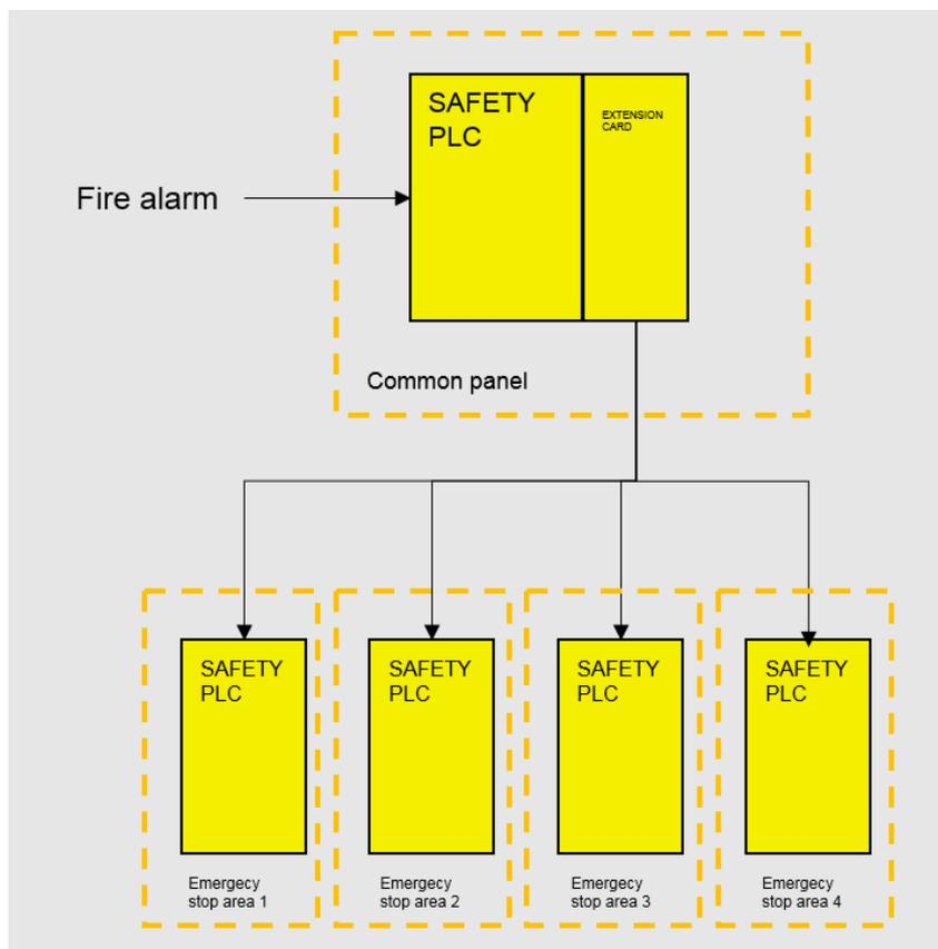
Figure 6. Technical principle of the common panel.
