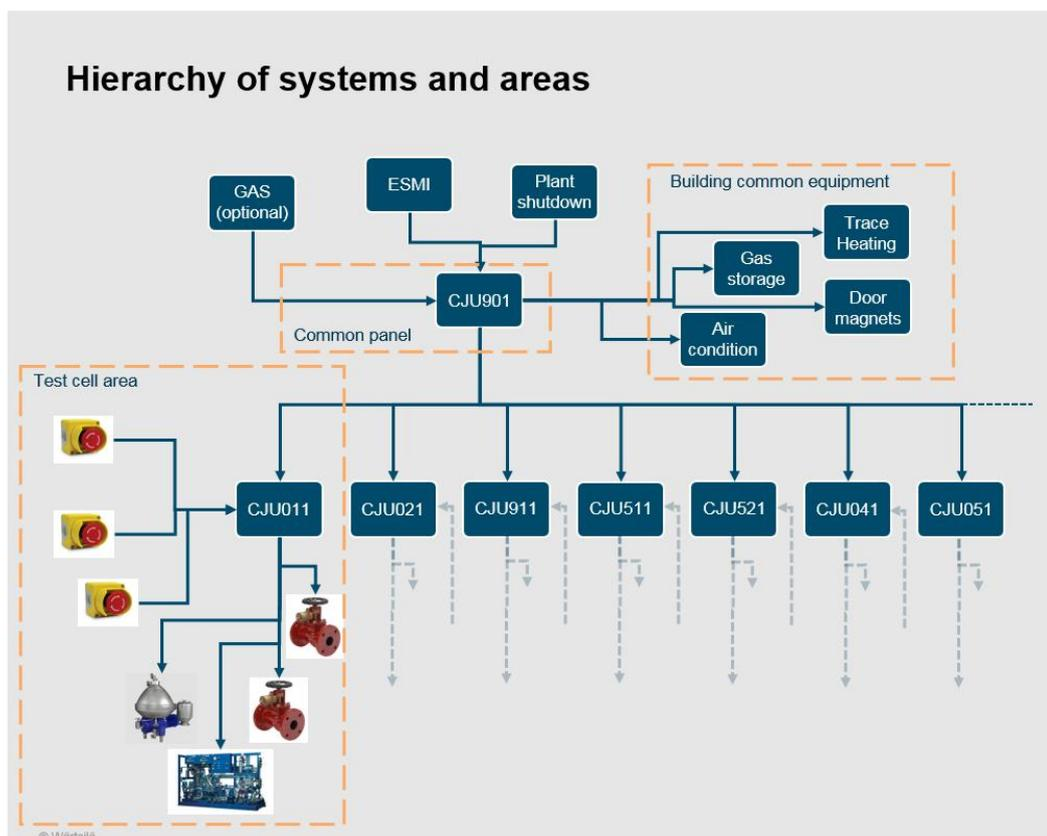
Figure 4. Principle of hierarchy in the emergency stop system.
