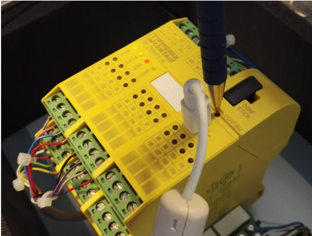
Figure 28. CONFIRM – button is located in a hole right above Mini USB port. The button can be used with a pen or a match. A small click is enough for confirming the new program downloaded on the safety PLC.
