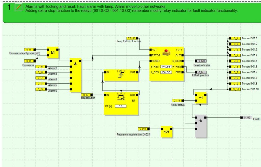
Figure 29. Main network on Common panel CJU901 program. The main network has all properties on build.
