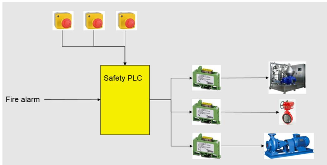
Figure 5. Technical principle of the emergency stop area.
