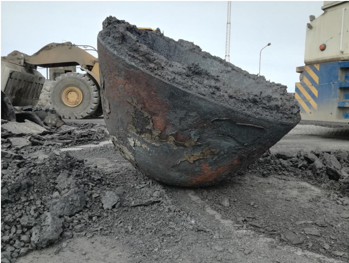
FIGURE 10. A lot of steel was tapped to the slag pot
