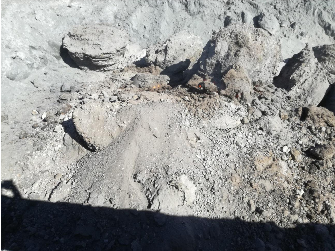
FIGURE 36. The desulphurisation slag dippings in their pit
