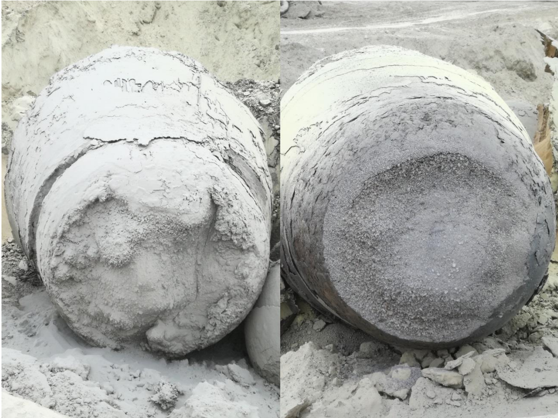
FIGURE 38. Emptied ladle slag blocks in which the protective LD slag stayed at the bottom, thus flat shape
