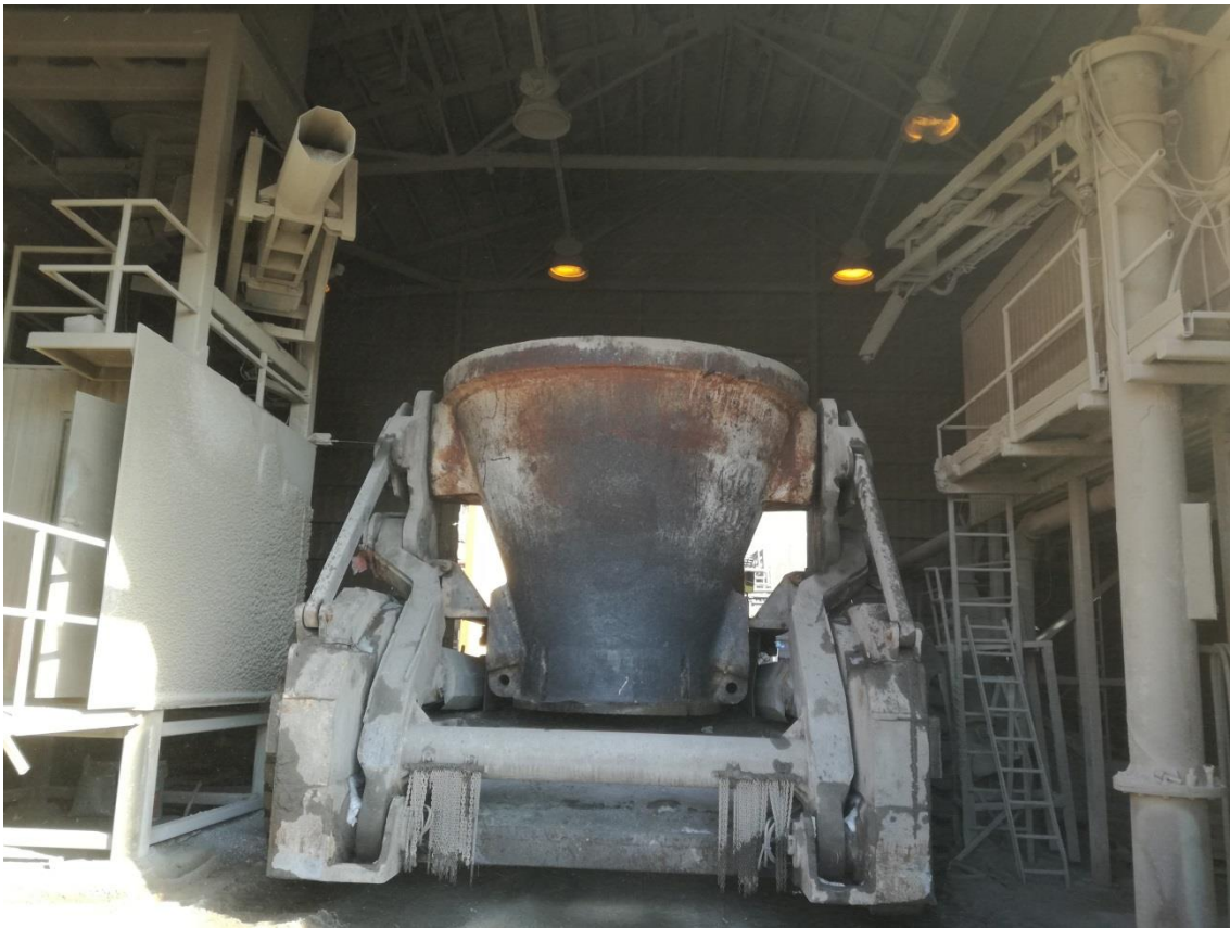
FIGURE 13. The slag pot carrier truck in the sanding station
