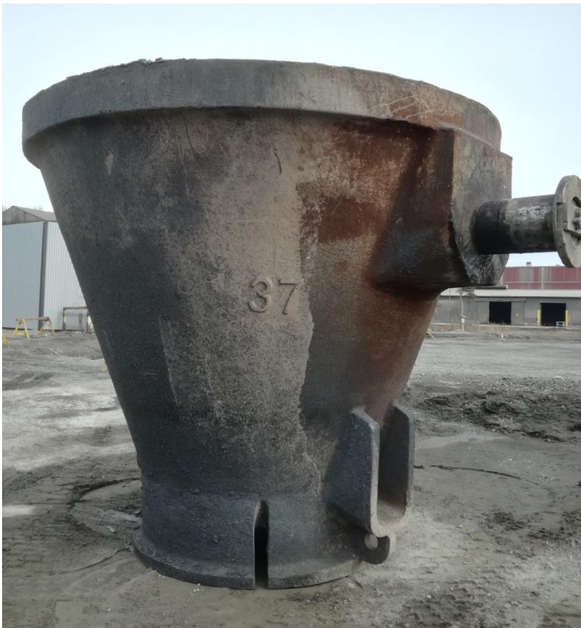
FIGURE 5. The slag pot used at the converters as the LD slag pot
