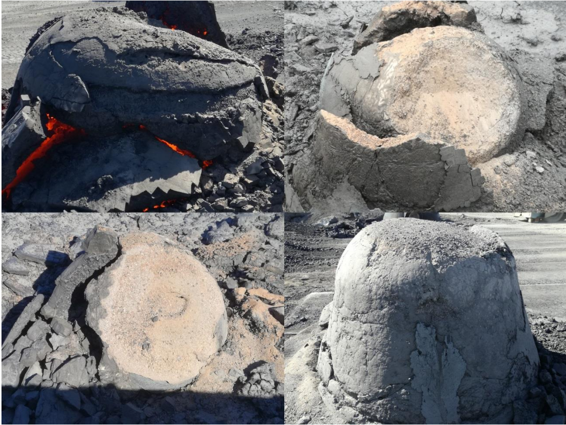
FIGURE 31. The LD slag stayed at the bottom of the LD pots as it should
