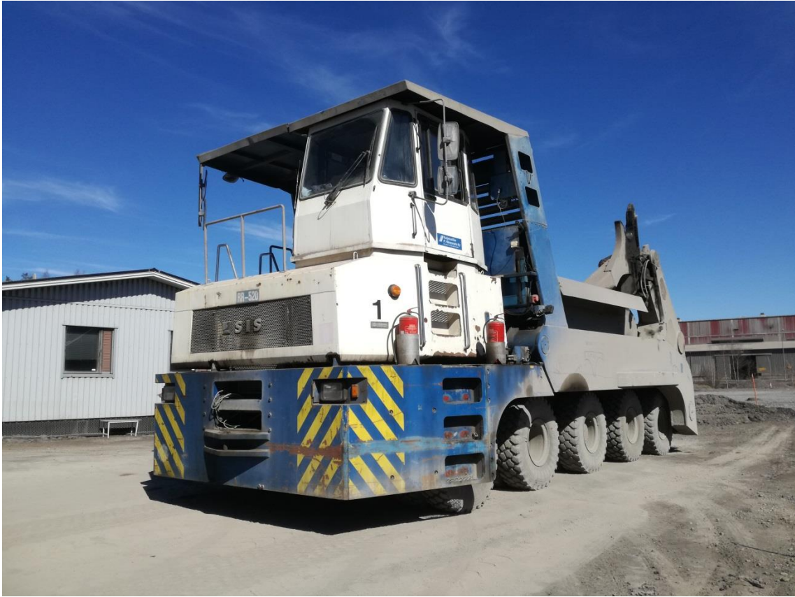
FIGURE 7. The slag pot carrier truck used to transport the LD slag pots
