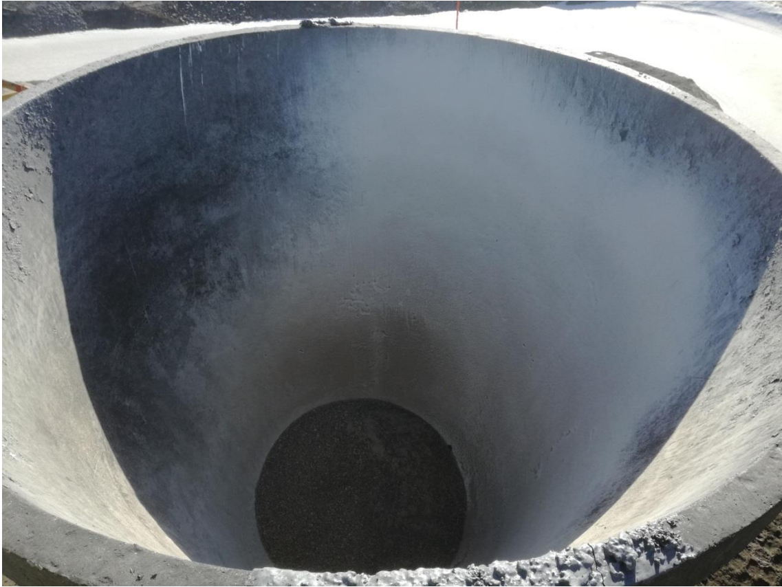
FIGURE 9. The slag pot with the lime suspension and the protective sand
