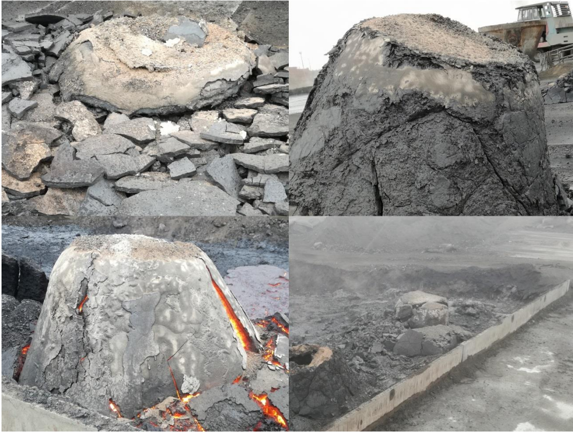
Figure 28. The LD slag stayed at its place in the bottom of the pots
