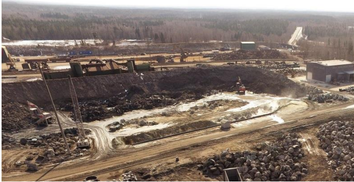
FIGURE 4. The dipping pit for the ladle slag
