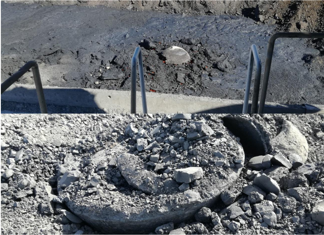
FIGURE 26. The LD slag has either been melted or pushed aside thus round shape
