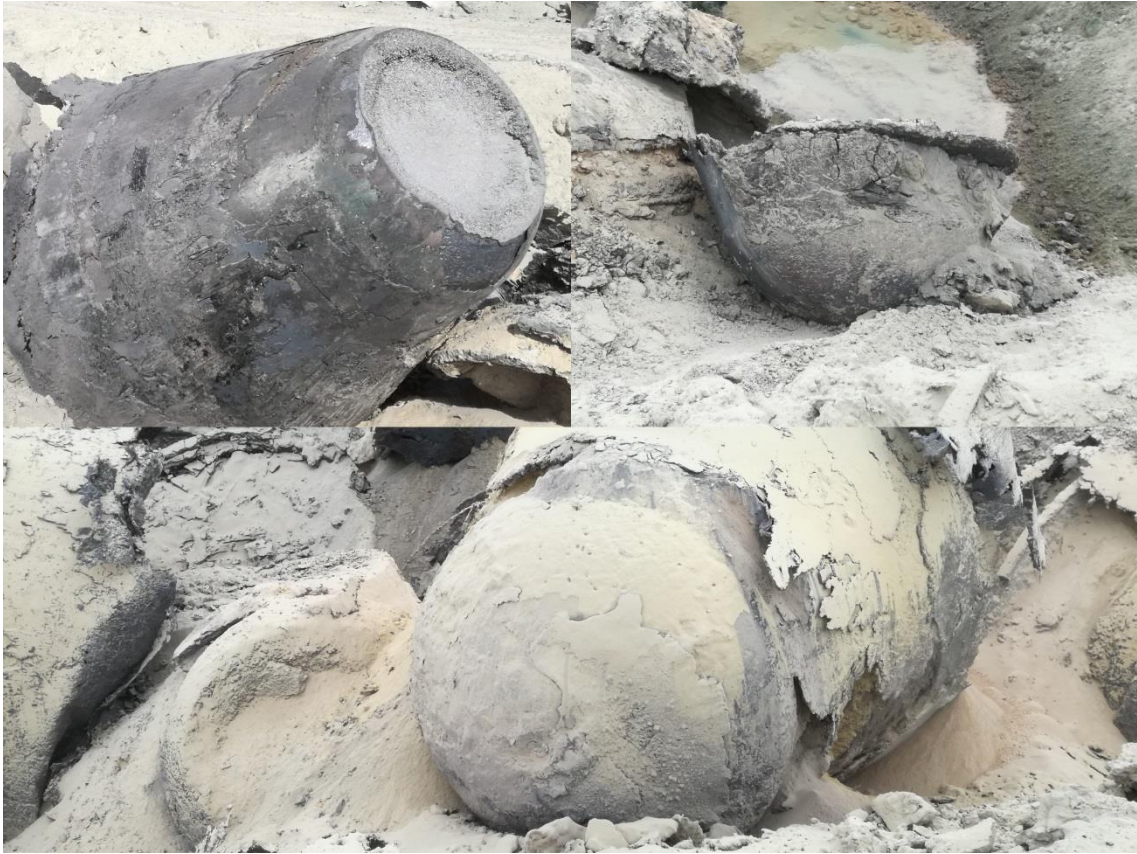
FIGURE 39. Emptied ladle slag, comparison between flat and round shaped bottoms
