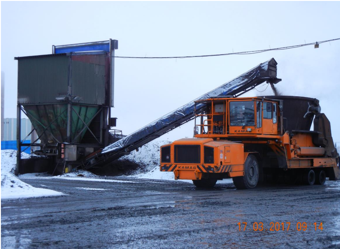
FIGURE 14. Approximately 150–200 kg of the protective sand is being fed to the melting shop's slag pot in Luleå (Virtala 2017)
