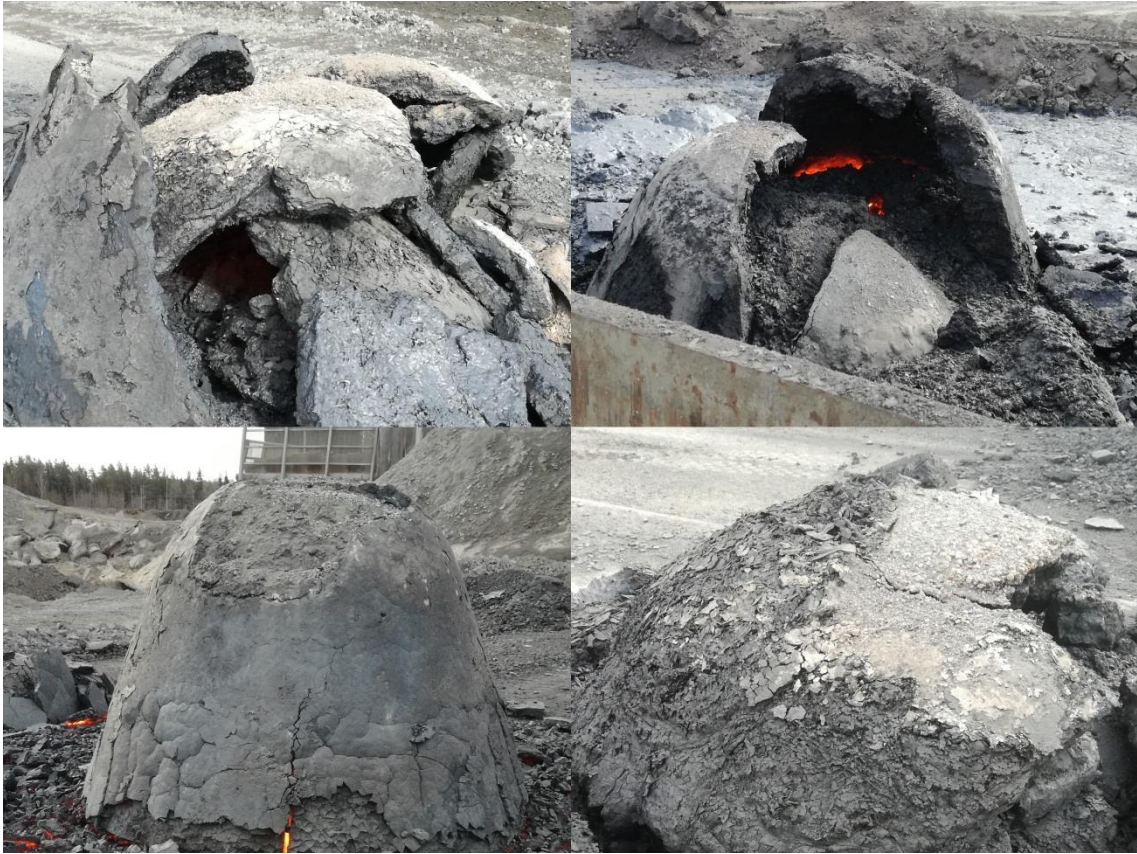
FIGURE 23. Some of the sand has been pushed aside thus the almost round shape
