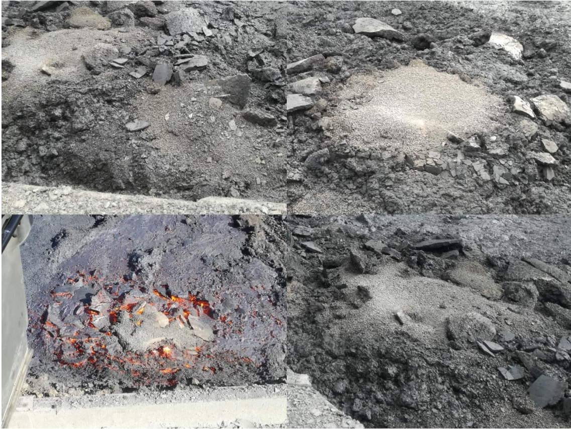
FIGURE 25. The large amount of the LD slag is clearly visible and pots emptied correctly
