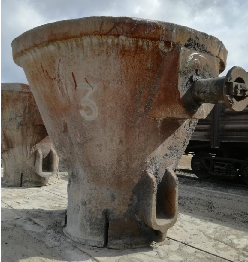
FIGURE 6. The slag pot used at the mixers as the desulphurisation slag pot
