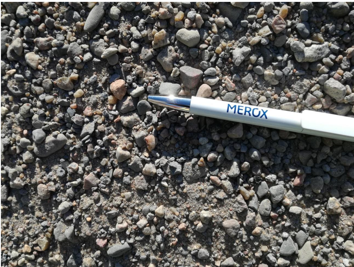
FIGURE 15. The natural sand 0–10 mm
