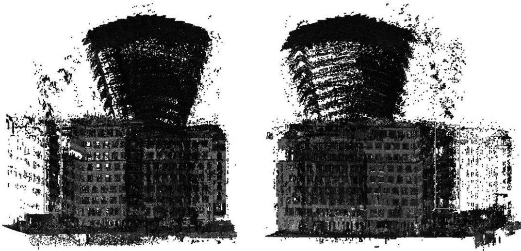
Figure 26 Occluded registered point cloud of Verbändehaus
