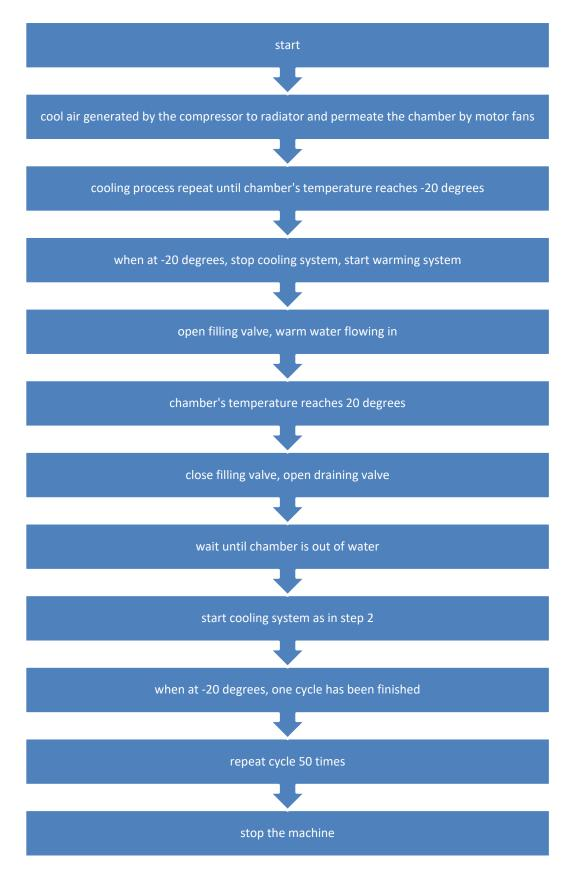
Figure 2. Working process by flowchart (chart created by the author)
