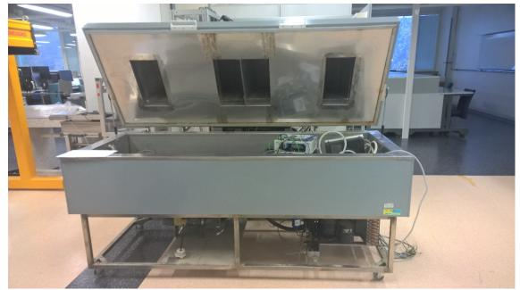
Figure 18. Exterior design of thermal cycling testing chamber (photograph taken by the author)
