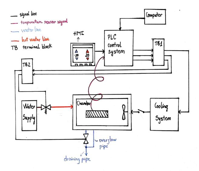
Figure 17. Thermal cycling testing machine connection diagram (diagram drawn by the author)
