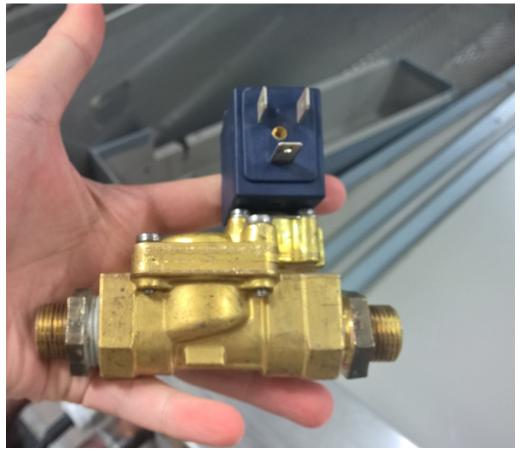
Figure 12. Old valve which needs to replace (photograph taken by the author)
