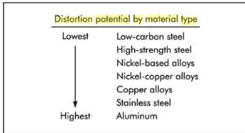
Figure 45: Distortion potential based on material type. (Nee 2010, 324)
