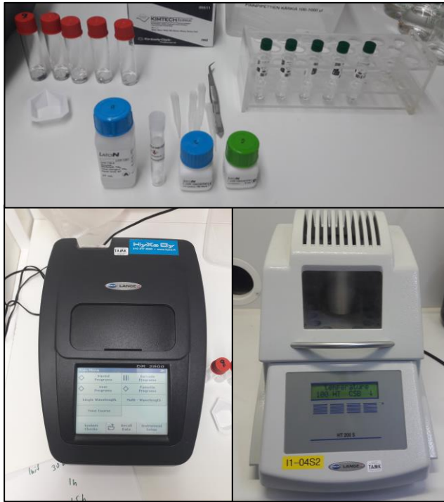
PICTURE 3. Devices and reagents required for HACH total nitrogen analysis.
