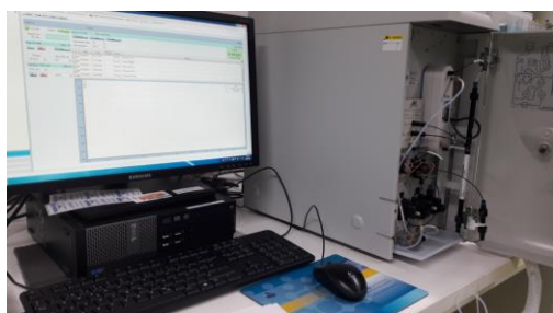
PICTURE 4. Ion chromatograph with a computer with Chromeleon software.
