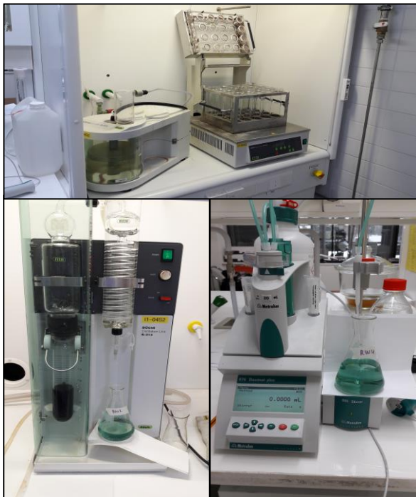
PICTURE 2. Set of apparatus required for TKN analysis.
