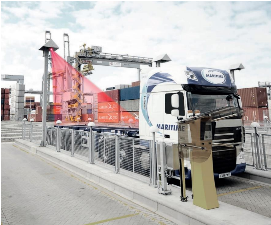
PICTURE 7. Laser measurement enables automated truck handling. (Kalmar 2014.)
