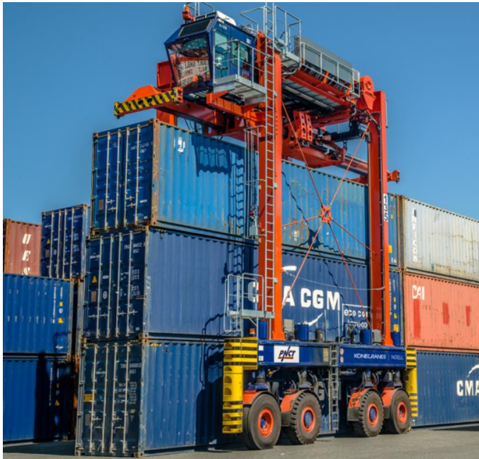
PICTURE 4. Straddle carriers are much higher than shuttle carriers. (Konecranes 2018.)
