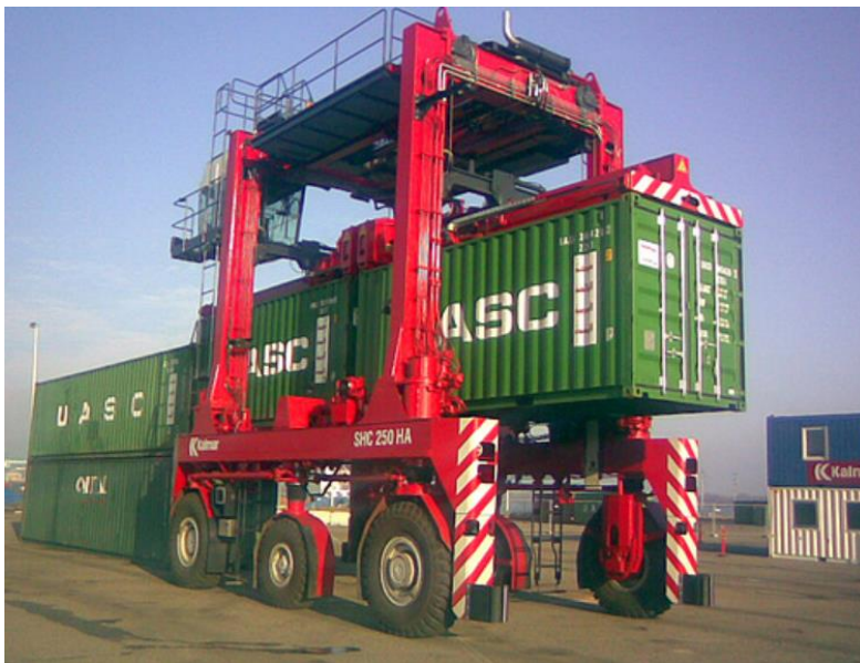
PICTURE 2. Kalmar shuttle carriers have a lifting capacity up to 50 tons. (SAE International 2008.)
