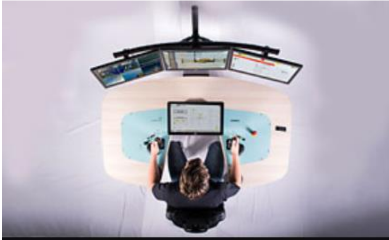
PICTURE 18. The screens should be mounted on a slight angle to expand the field of vision (Siemens 2018.).
