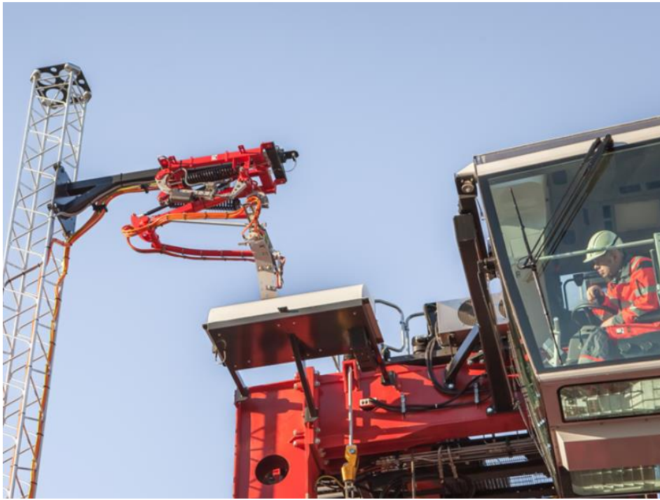
PICTURE 3. Kalmar FastCharge charging station enables the shuttle carrier to operate continuously. (Kalmar 2017a.)
