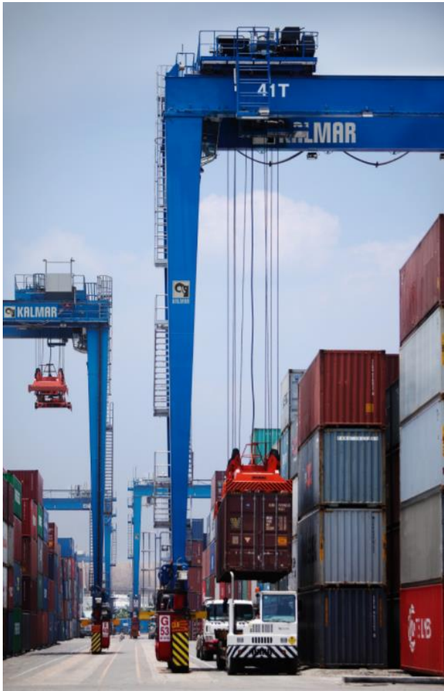
PICTURE 10. Location of the truck lane in RTG operation. (Kalmar 2016.)
