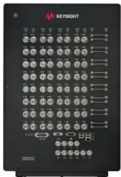
FIGURE 3. Anite Prosim F32 Channel Emulator (2).
