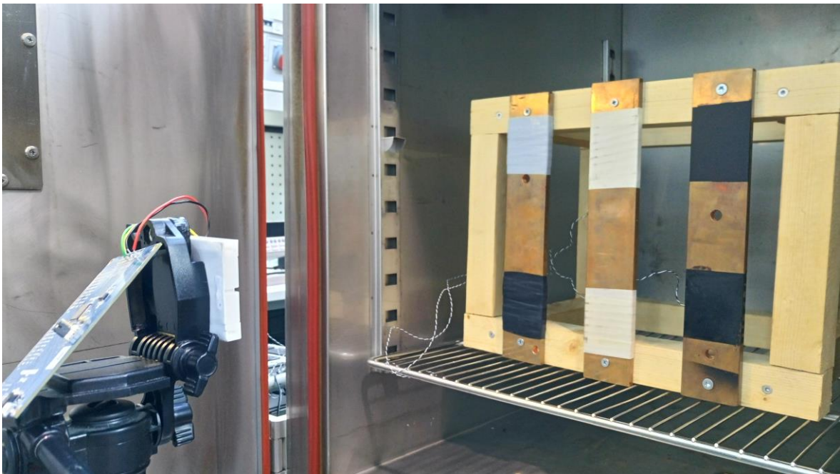
Figure 11 - The IR sensor is mounted to measure temperatures from the bus bar rig
