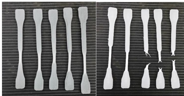
Figure 34. Printed tensile specimens of rHDPE and pristine HDPE (from left to right)
