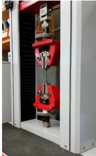
Figure 22. Material testing machine, Testometric M 350- 5CT, Arcada 2018
