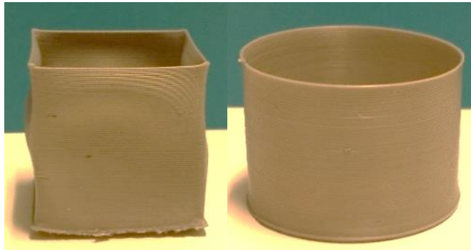
Figure 38. rHDPE printed samples of hollow cube and cylinder
