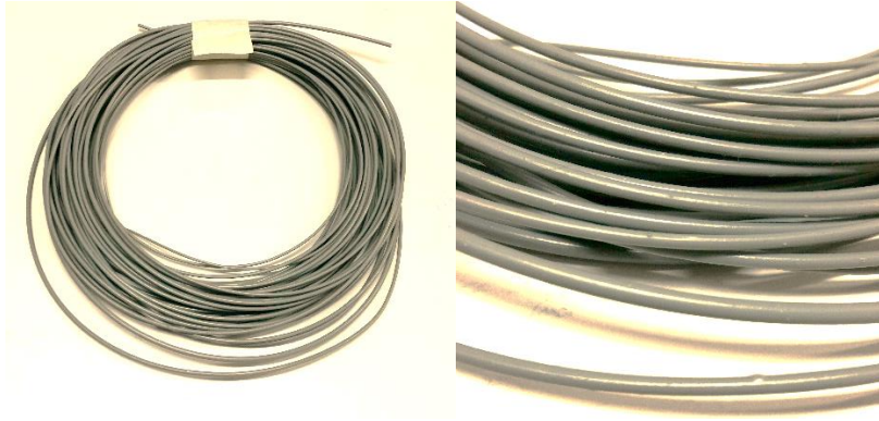
Figure 28. Produced filament from rHDPE
