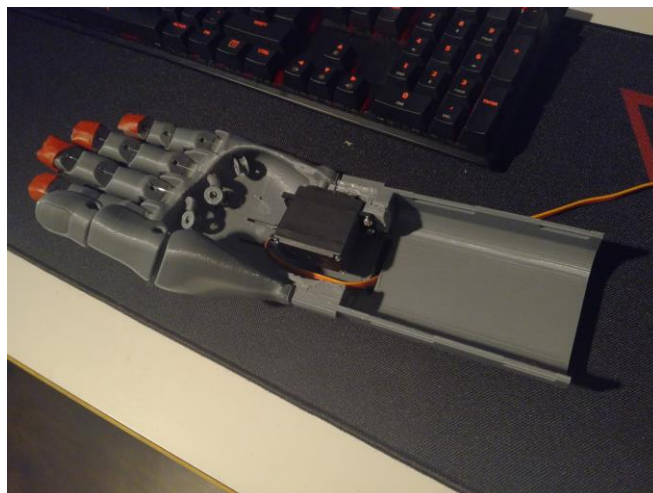
Figure 19: Hand and gauntlet assemble with PWM motor
