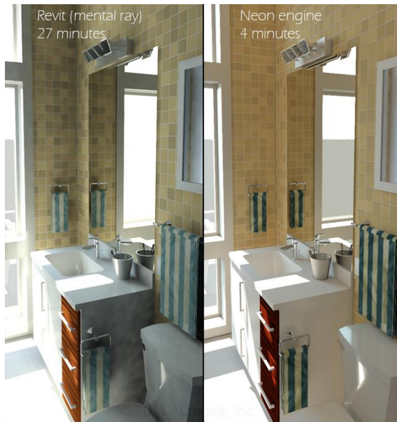
Figure 4: Comparison between Revit rendering tool and cloud based Neon engine (Cloud Rendering, n.d.)
