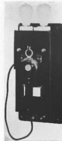
Sending Station Single Hand Type Transmitter and 110-Volt D. C. Control Board
