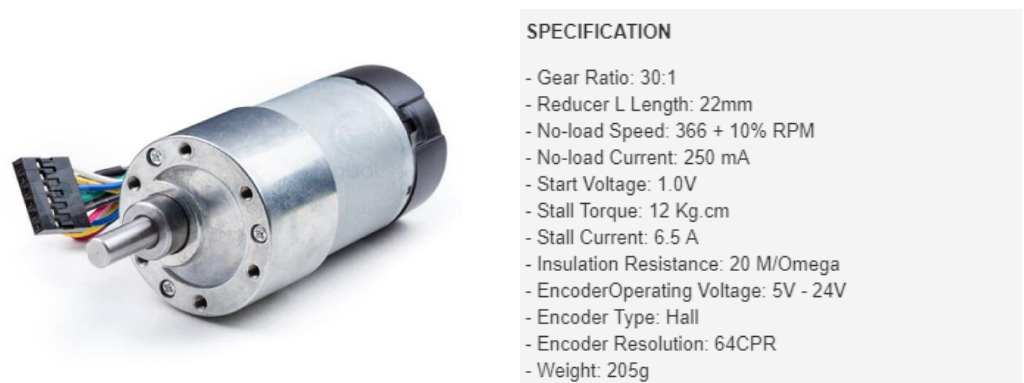
Figure 12. 12V motor with hall quadrature sensor encoder (product, n.d.)
