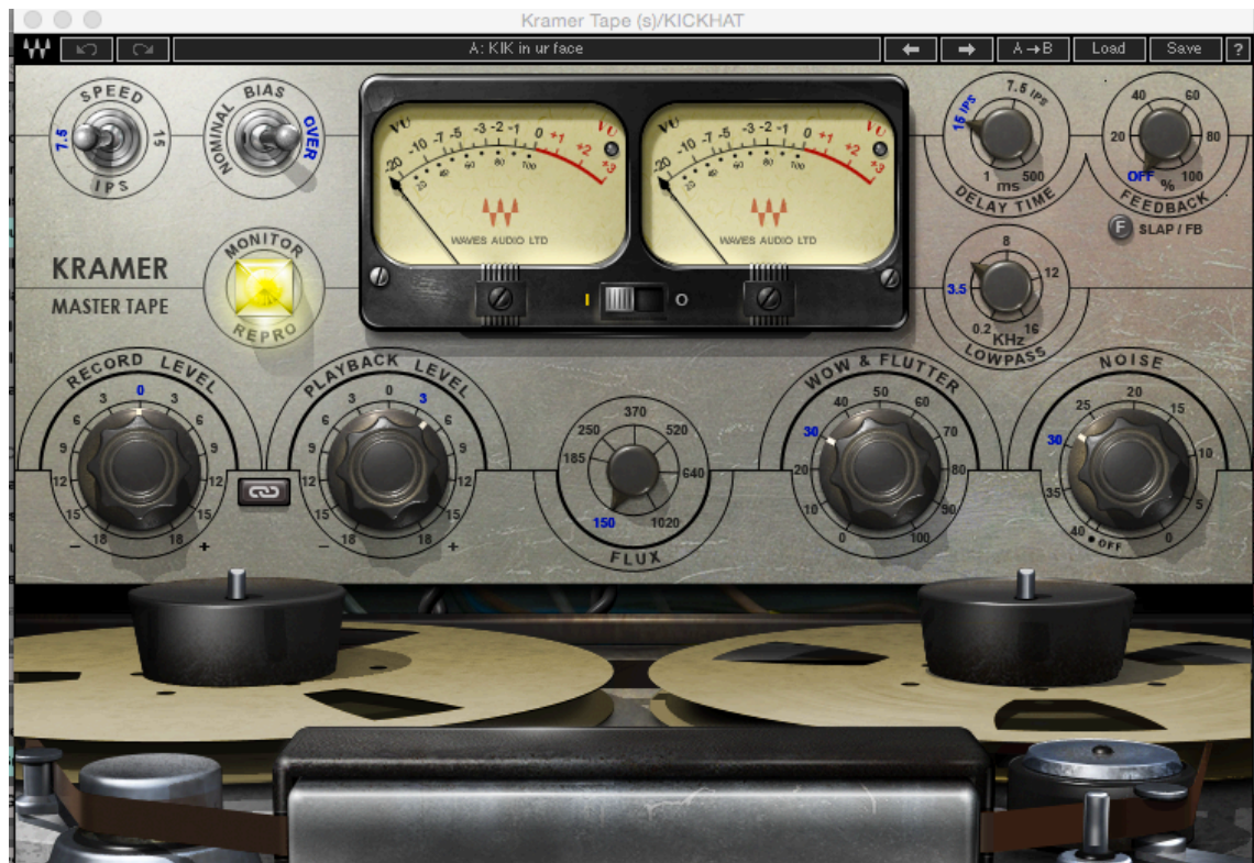
PICTURE 10: Kramer Tape Plugin Adding Saturation to a Kick Drum (Mika Kurvinen 2018)
