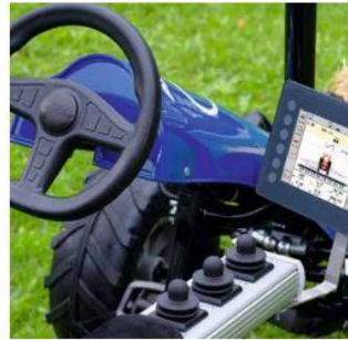
Figure 2: ISOBUS AUX-N operating console integrated into the armrest
