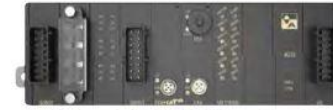
Figure 4: M20i as a gateway for fast ISOBUS retrofitting of existing control systems
