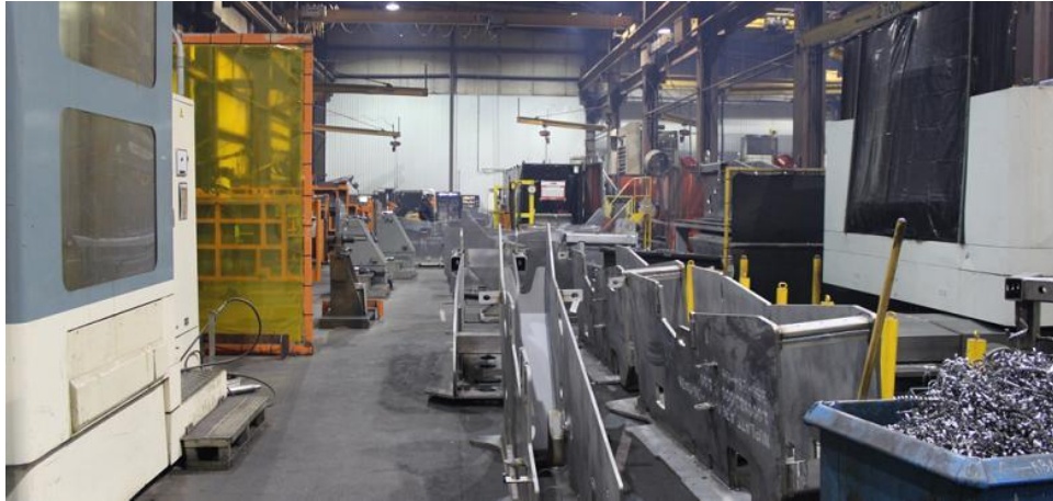
Figure 6. Before lean, parts waiting for the next process in queue – push system. (Heston T., 2014.)
