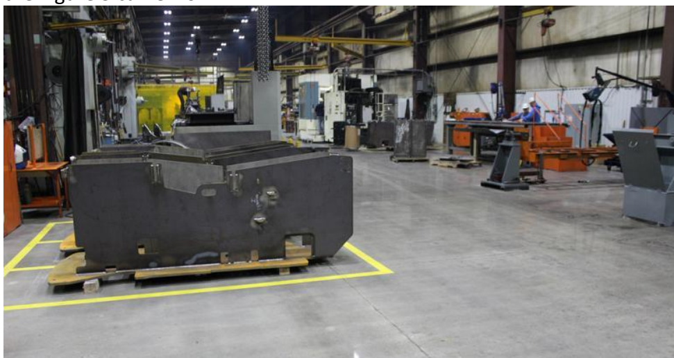
Figure 5. Lines marking the work-in-progress areas and shined floor. (Heston T., 2014.)
