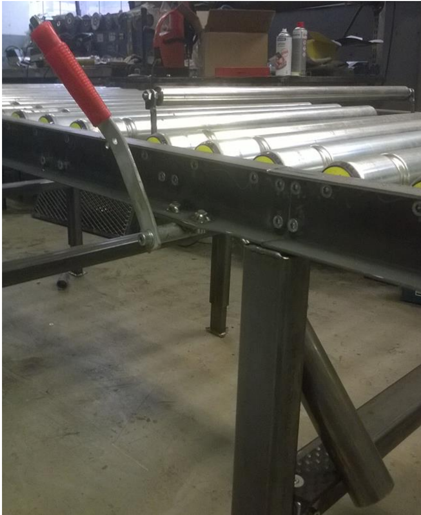
PICTURE 17. The brake installed on the prototype. The counterweight has a separate stopper to absorb impact. (Härkönen 2018)
