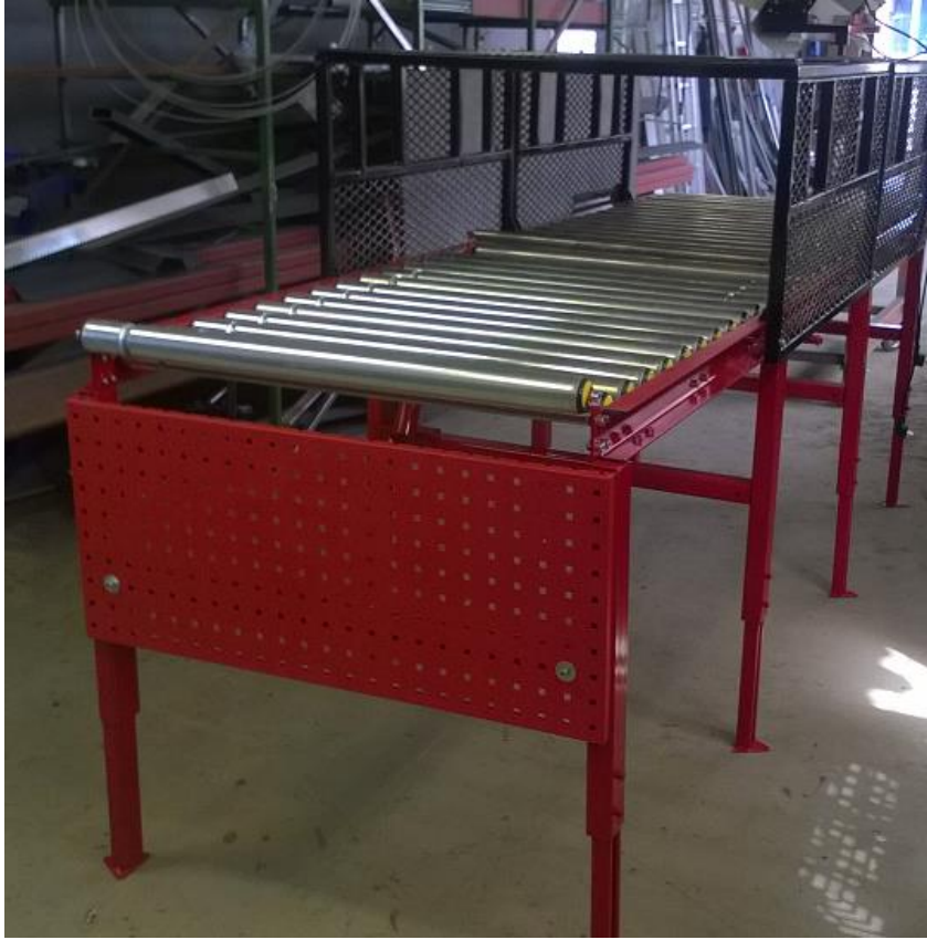
PICTURE 18. The tool wall at the end of the conveyor can be used to hold tools for the next work phase, like balancing (Härkönen 2018)
