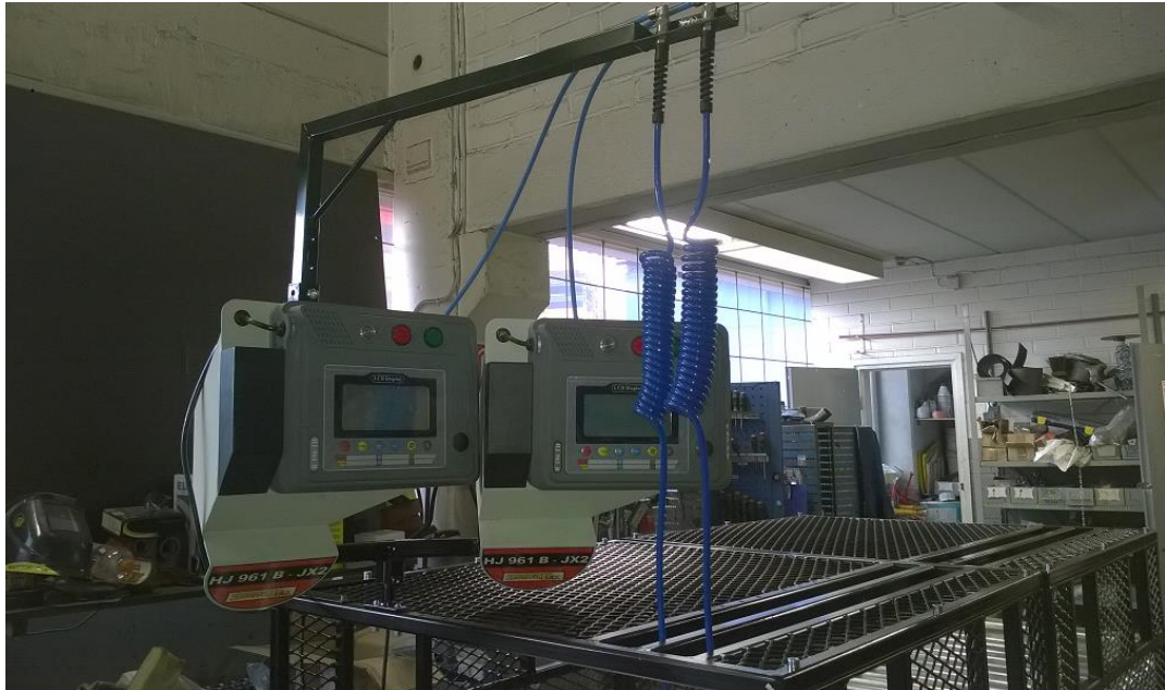
PICTURE 15. The inflation robot mount rotates and is fixed in place by a bolt. The prototype is assembled as a mirror image of the 3D model, which is possible due to the modular nature of the product. (Härkönen 2018)
